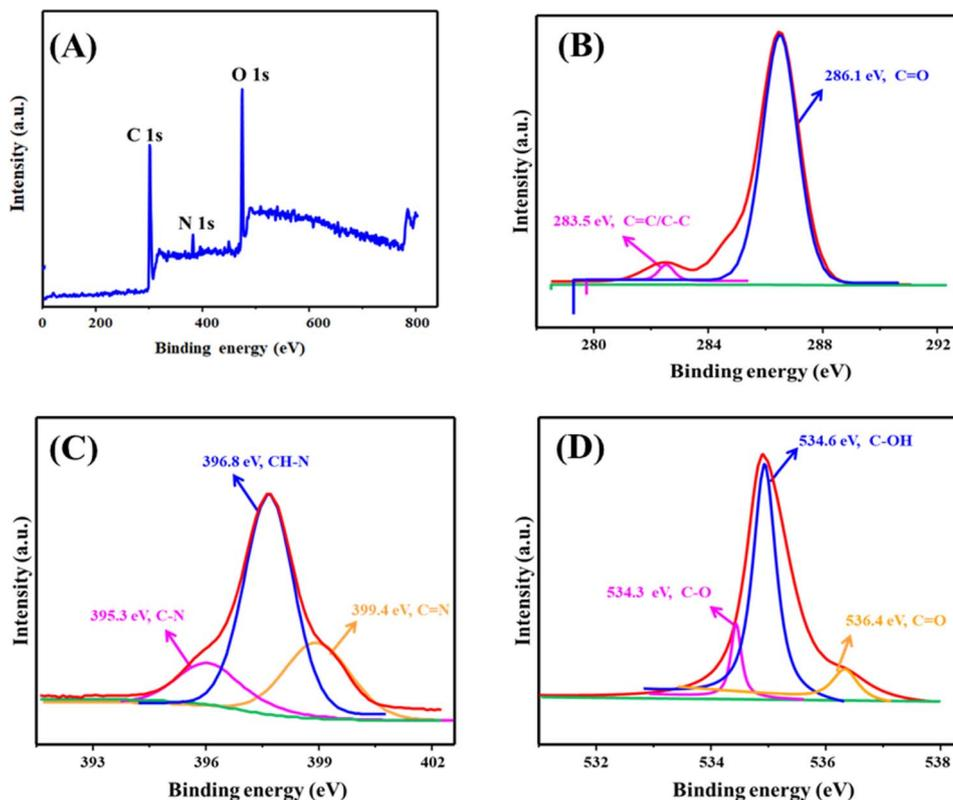
Fig. 2 (A) Full XPS survey of plastic syringe -derived CDs; (B–D) deconvoluted spectra of C 1s, N 1s, and O 1s, respectively.
