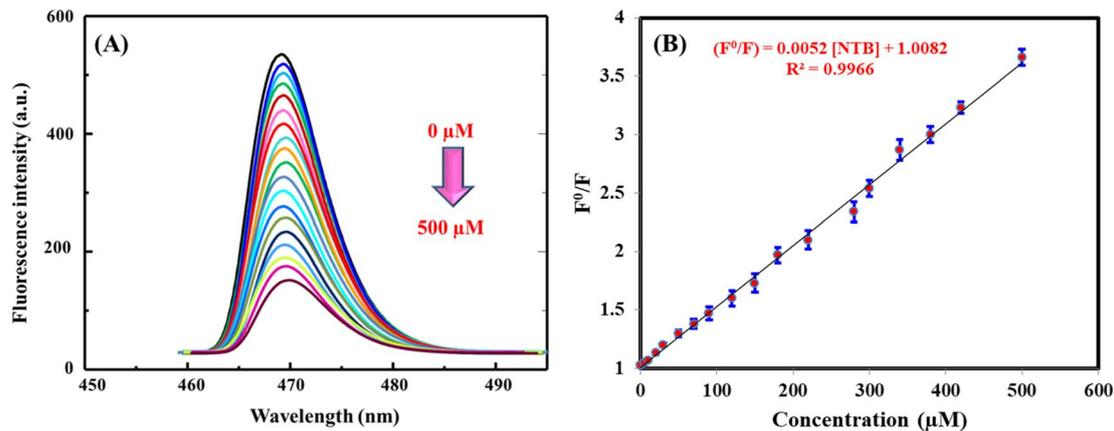
Fig. 3 (A) Fluorescence responses of CDs upon addition NTB (0–500  $\mu\text{M}$ ) and (B) corresponding calibration plot. Conditions are CDs' concentration is  $100 \mu\text{g mL}^{-1}$ , pH 7.4, and incubation time is 1 min.
