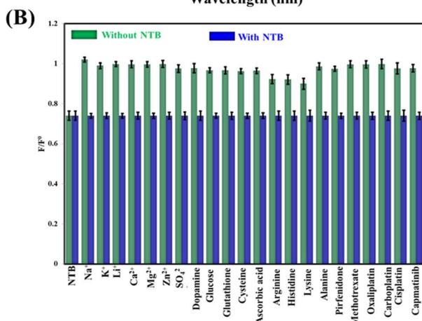
Fig. 4 Fluorescence responses (A) and corresponding bar diagram (B) of the CDs-based probe in the presence (anti-interference) and absence (selectivity) of 50  $\mu\text{M}$  NTB and ten-fold of interfering species (ions, biomolecules, anti-cancer drugs). Conditions are CDs' concentration is 100  $\mu\text{g mL}^{-1}$ , pH 7.4, and incubation time is 1 min.
