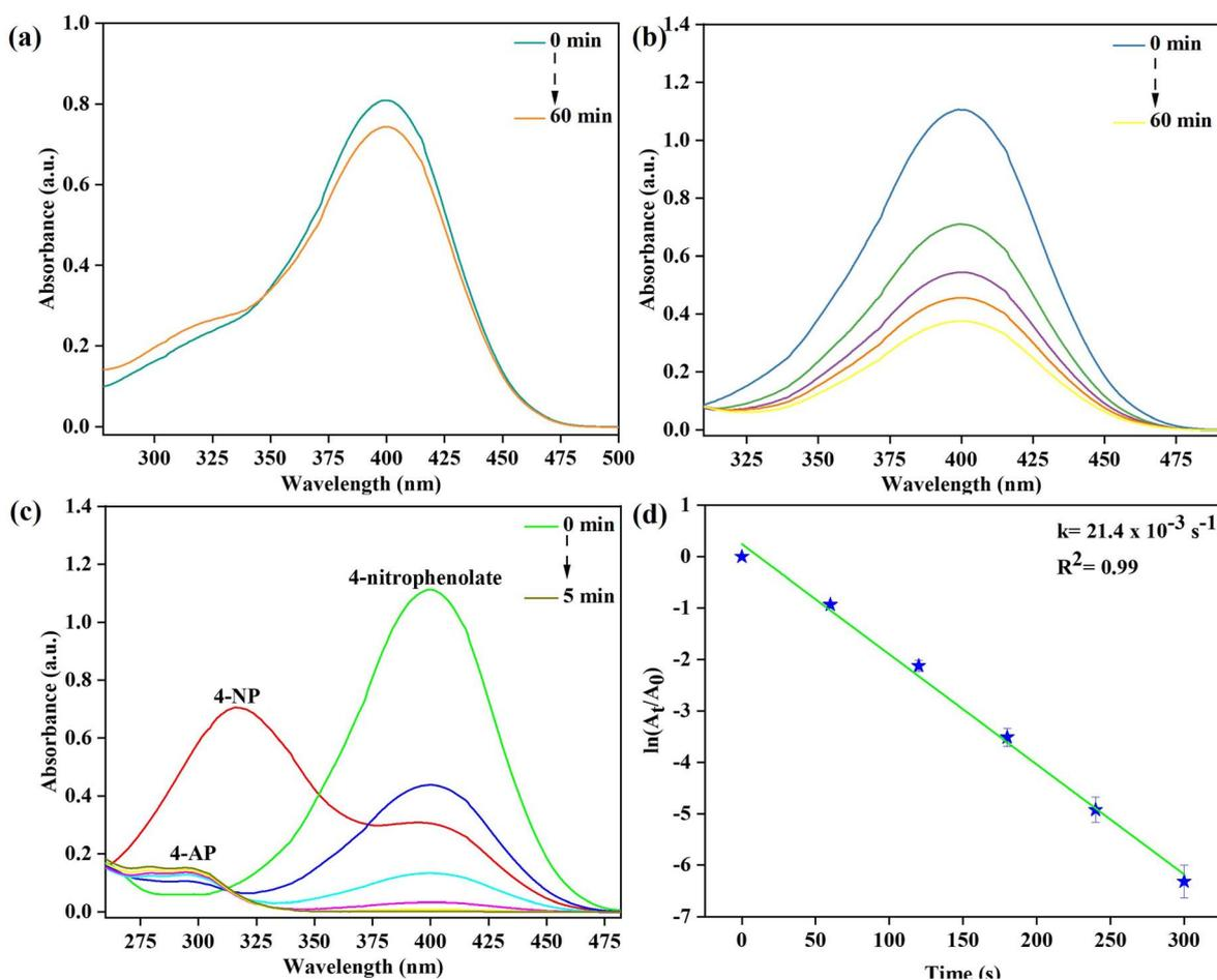
**Fig. 6** UV-visible spectra illustrating the reduction of 4-NP under various conditions (a) in the absence of  $\text{NaBH}_4$ , (b) without  $\text{Ag}@CS\text{-}BCN$  nanohybrid, (c) in the presence of both  $\text{NaBH}_4$  and  $\text{Ag}@CS\text{-}BCN$  nanohybrid under optimised conditions and (d) the corresponding kinetic plot of  $\ln(A_t/A_0)$  versus time.
