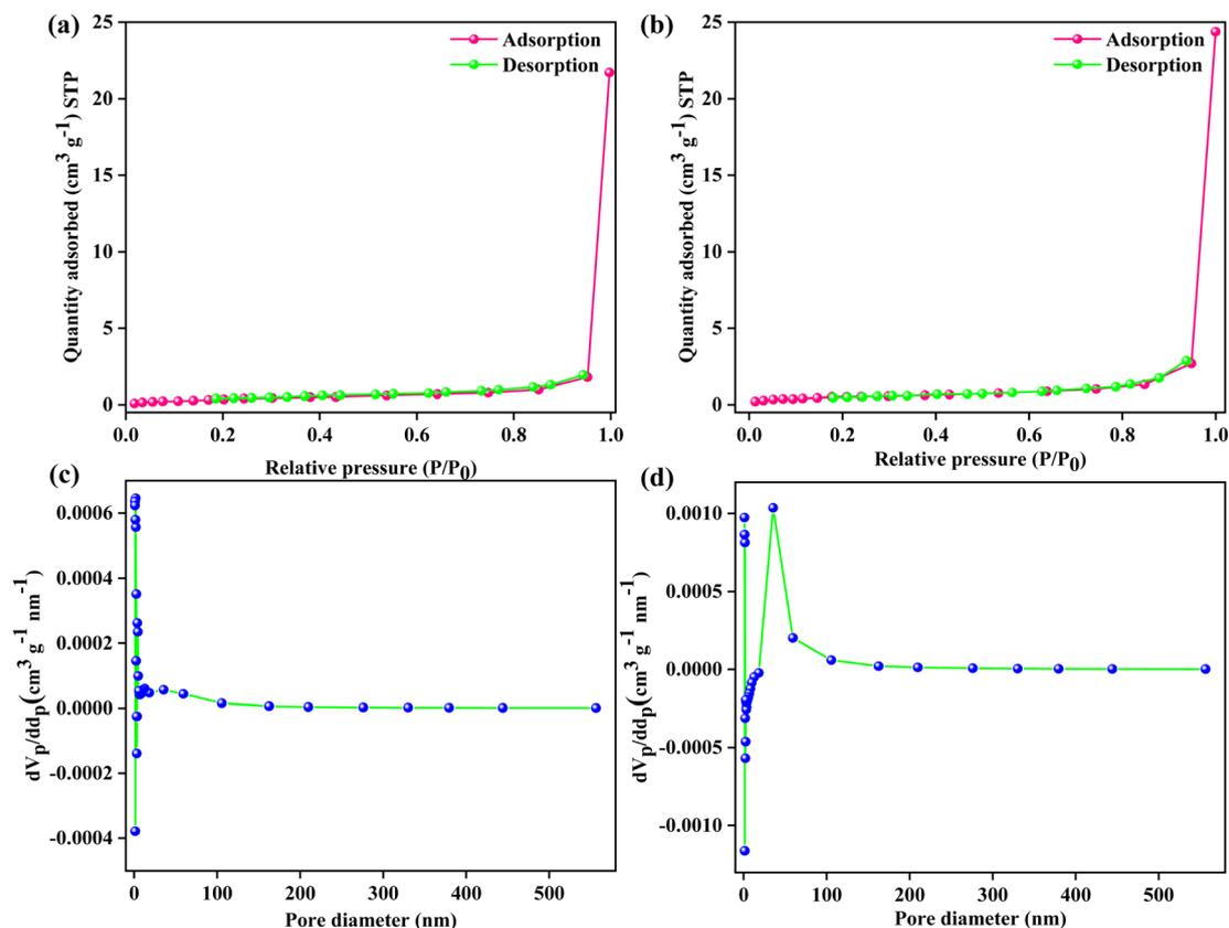
Fig. 5 Nitrogen adsorption–desorption isotherm curves for (a) CS–BCN and (b) Ag@CS–BCN nanohybrid; BJH pore size distribution plot of (c) CS–BCN and (d) Ag@CS–BCN nanohybrid.
