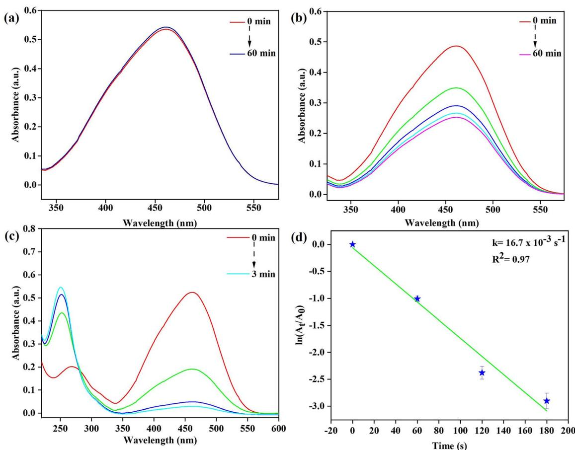
**Fig. 7** UV-visible spectra demonstrating the reduction and degradation of MO under various conditions: (a) in the absence of NaBH<sub>4</sub>, (b) without Ag@CS-BCN nano hybrid, (c) in the presence of both NaBH<sub>4</sub> and Ag@CS-BCN nano hybrid, and (d) the corresponding kinetic plot of  $\ln(A_t/A_0)$  versus time.
