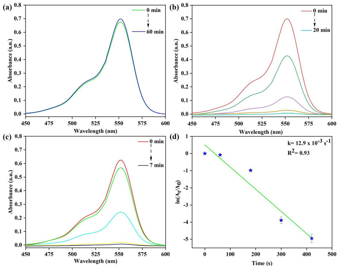
Fig. 8 UV-visible spectra demonstrating the reduction and degradation of RhB to leuco RhB under various conditions in the absence of: (a)  $\text{NaBH}_4$ , (b)  $\text{Ag}@CS\text{-}BCN$  nanohybrid, and (c) in the presence of both  $\text{NaBH}_4$  and  $\text{Ag}@CS\text{-}BCN$  nanohybrid, and (d) the corresponding kinetic plot of  $\ln(A_t/A_0)$  versus time.
