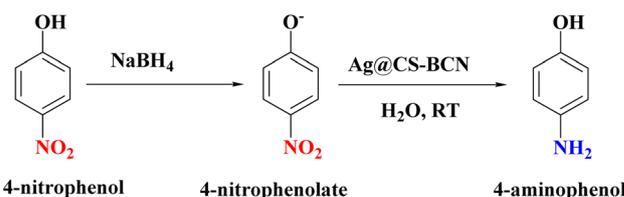
Scheme 2 The catalytic activity of Ag@CS–BCN nanohybrid in the reduction of 4-NP to 4-AP using NaBH<sub>4</sub> under ambient conditions.
