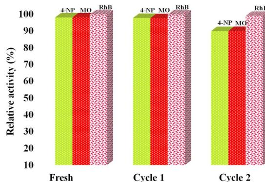
**Fig. 9** Recyclability study for reducing 4-NP and degradation of MO and RhB dyes.
