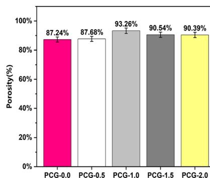
Fig. 5 Porosity of PLA/CPP/GO composite scaffolds with different GO contents. No statistically significant differences were found between the groups ( $p > 0.05$ , one-way ANOVA). All data are presented as mean  $\pm$  standard deviation ( $n \geq 7$ ).
