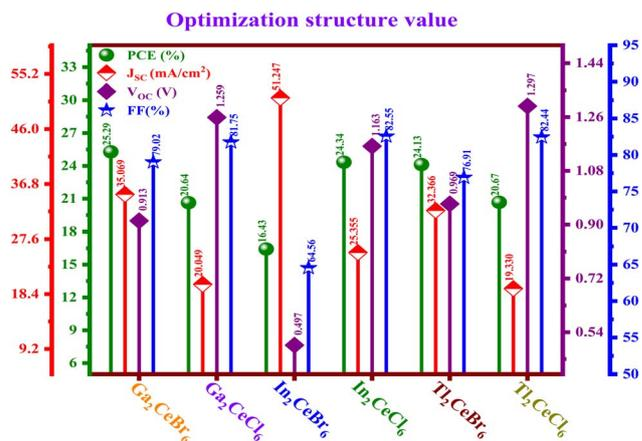
Fig. 28 Comparison of  $V_{\text{OC}}$ ,  $J_{\text{SC}}$ , FF, and PCE for  $\text{Ga}_2\text{CeBr}_6$ ,  $\text{Ga}_2\text{CeCl}_6$ ,  $\text{In}_2\text{CeBr}_6$ ,  $\text{In}_2\text{CeCl}_6$ ,  $\text{Tl}_2\text{CeBr}_6$ , and  $\text{Tl}_2\text{CeCl}_6$  absorber-based solar cells.
