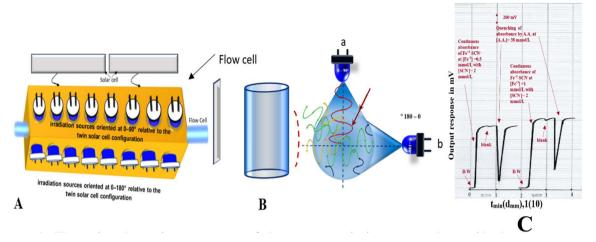
Fig. 1 Illustrating the main components of the spectroscopic instrument along with the measurement configuration: (A) measurement cell, (B) illuminated area by: (a) source at  $0-90^\circ$ , (b) source at 0-180, (C) real profile measured responses obtained from the chart recorder (T: time in minute, d: distance in millimeter).
