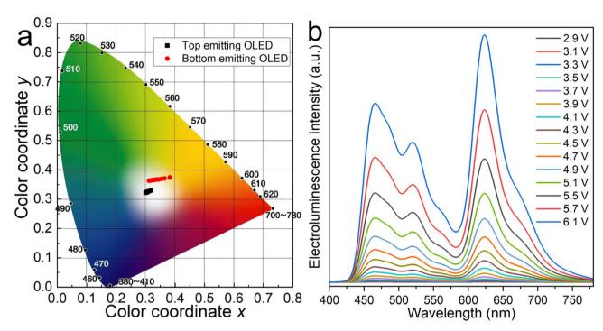
Fig. 6 (a) Chromaticity coordinates of top- and bottom-emitting OLEDs at different working voltages within the range of 2.8–6.2 V; (b) electroluminescence emission spectra of top-emitting OLED at different working voltages.
