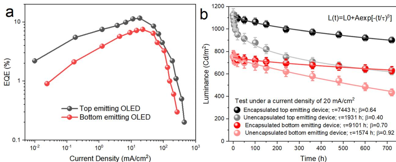
Fig. 4 (a) EQE of top- and bottom-emitting OLED devices. (b) Stability of the encapsulated and unencapsulated top- and bottom-emitting devices. Sample size is approximately 1.5 mm  $\times$  1.5 mm, the temperature is 25  $^{\circ}$ C, and the humidity is 70%.
