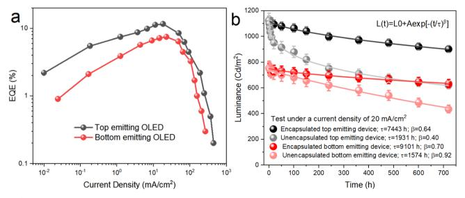
Fig. 4 (a) EQE of top- and bottom-emitting OLED devices. (b) Stability of the encapsulated and unencapsulated top- and bottom-emitting devices. Sample size is approximately 1.5 mm  $\times$  1.5 mm, the temperature is 25 °C, and the humidity is 70%.
