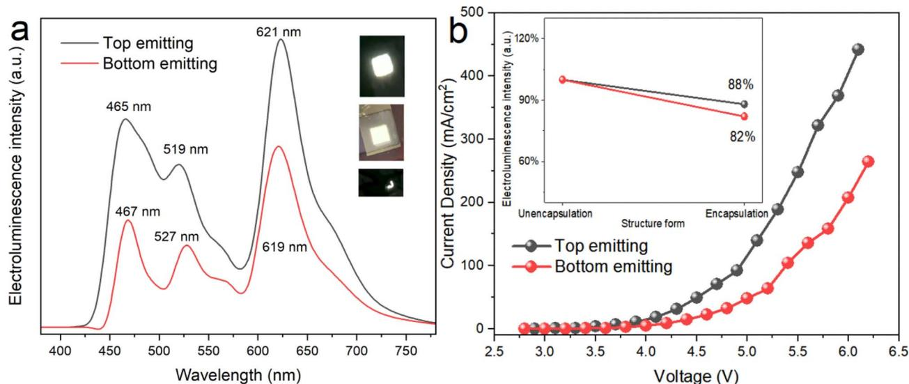
Fig. 3 (a) Electroluminescence emission spectra of top- and bottom-emitting OLED devices. (b) Current density–voltage ( $J$ – $V$ ) curves of top- and bottom-emitting OLED devices. The illustrations show illuminated encapsulated devices and the pressure test.
