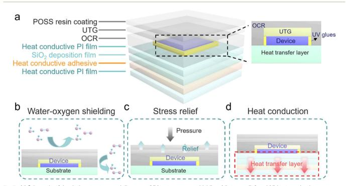
Fig. 7 (a) Schematic of the device structure, and diagrams of (b) water-oxygen shielding, (c) stress relief, and (d) heat conduction.
