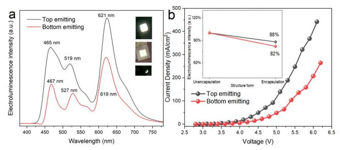
Fig. 3 (a) Electroluminescence emission spectra of top- and bottom-emitting OLED devices. (b) Current density-voltage (J-V) curves of top- and bottom-emitting OLED devices. The illustrations show illuminated encapsulated devices and the pressure test.
