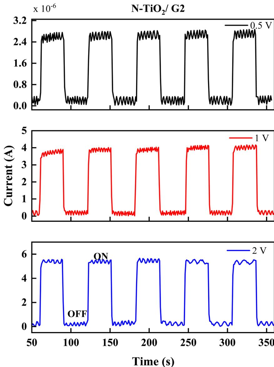
Fig. 13 The photodetection properties of a high concentration of graphene-supported N-TiO<sub>2</sub> at 0.5 V, 1 V and 2 V bias voltage.
