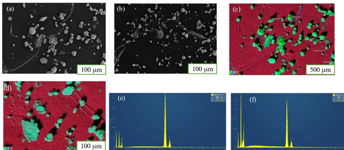
Fig. 3 The SEM mapped images and EDX spectra of nitrogenated  $\text{TiO}_2$  and graphene-supported  $\text{N-TiO}_2$ . (a)  $\text{N-TiO}_2$  (b) graphene supported  $\text{N-TiO}_2$  (c) and (d) mapped images of pristine and graphene supported  $\text{N-TiO}_2$  (e) and (f) EDX spectra of  $\text{N-TiO}_2$  and graphene supported  $\text{N-TiO}_2$ .
