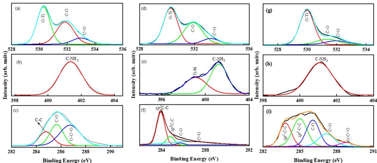
Fig. 8 The XPS spectra for pristine and graphene supported N-TiO<sub>2</sub> showing the elemental core levels. (a)–(c) pristine N-TiO<sub>2</sub> (d)–(f) NTiO<sub>2</sub>/G1 (g)–(i) N-TiO<sub>2</sub>/G2.
