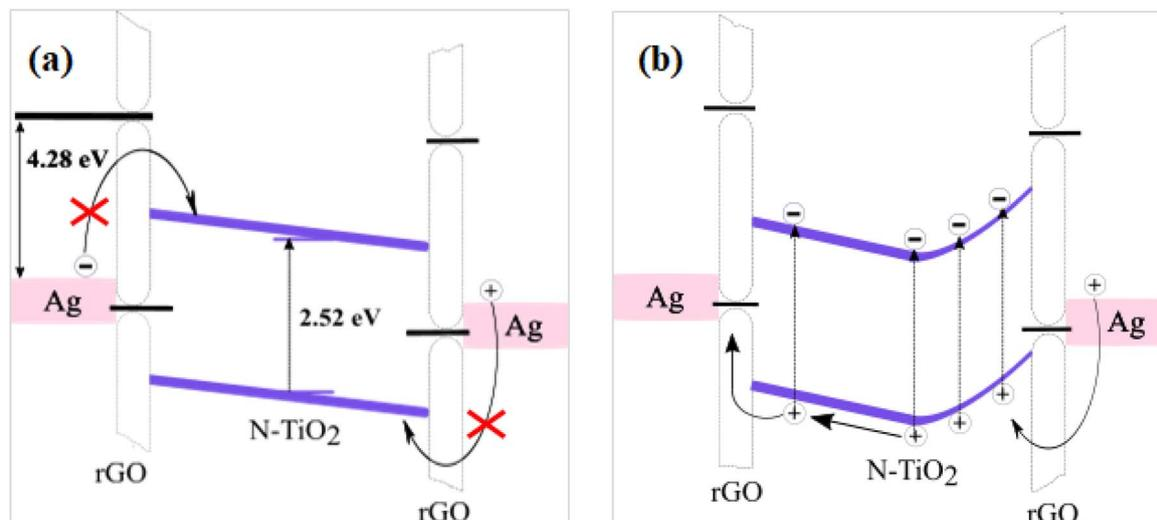
Fig. 15 The band alignment diagram for N-TiO<sub>2</sub>-supported graphene showing the charge transport properties. (a) The transfer of charges from Ag contacts to the active materials and (b) active material to the Ag contact.
