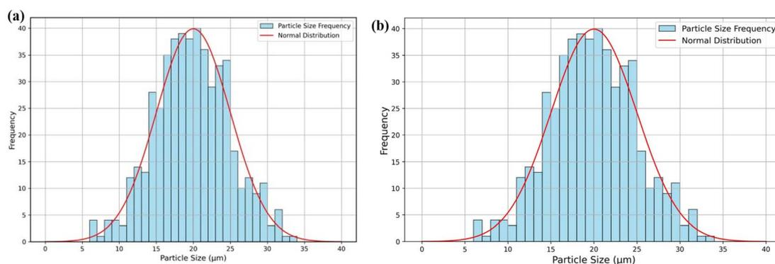
Fig. 4 Particle size distribution of (a) nitrogenated  $\text{TiO}_2$  and (b) graphene supported  $\text{N-TiO}_2$ .
