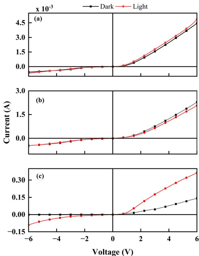
Fig. 10 Photoconductivity properties of pristine (a–c) graphene-supported N-TiO<sub>2</sub>/G.
