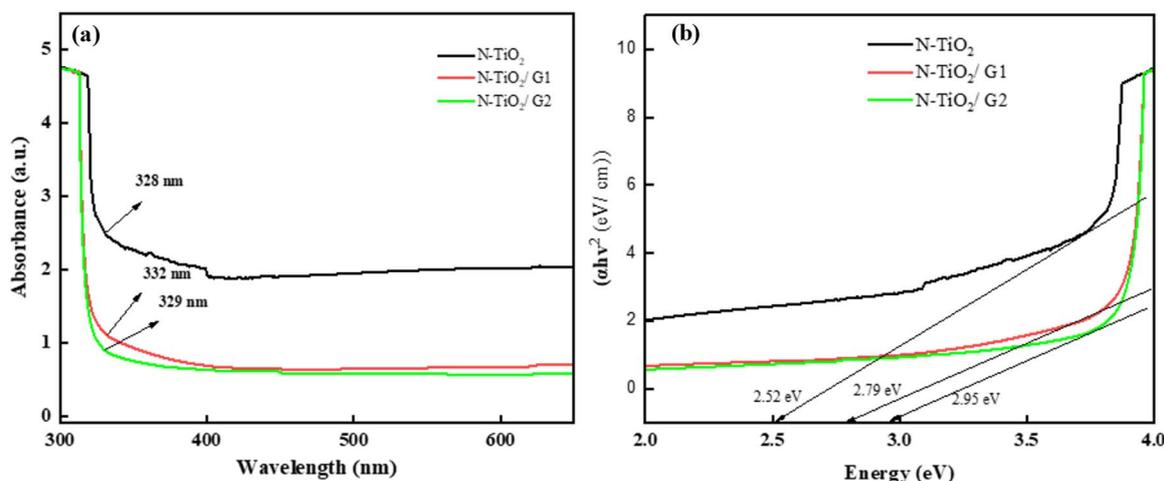
Fig. 6 (a) The UV-vis spectra and (b) Tauc plot of N-TiO<sub>2</sub> and graphene-supported N-TiO<sub>2</sub>.
