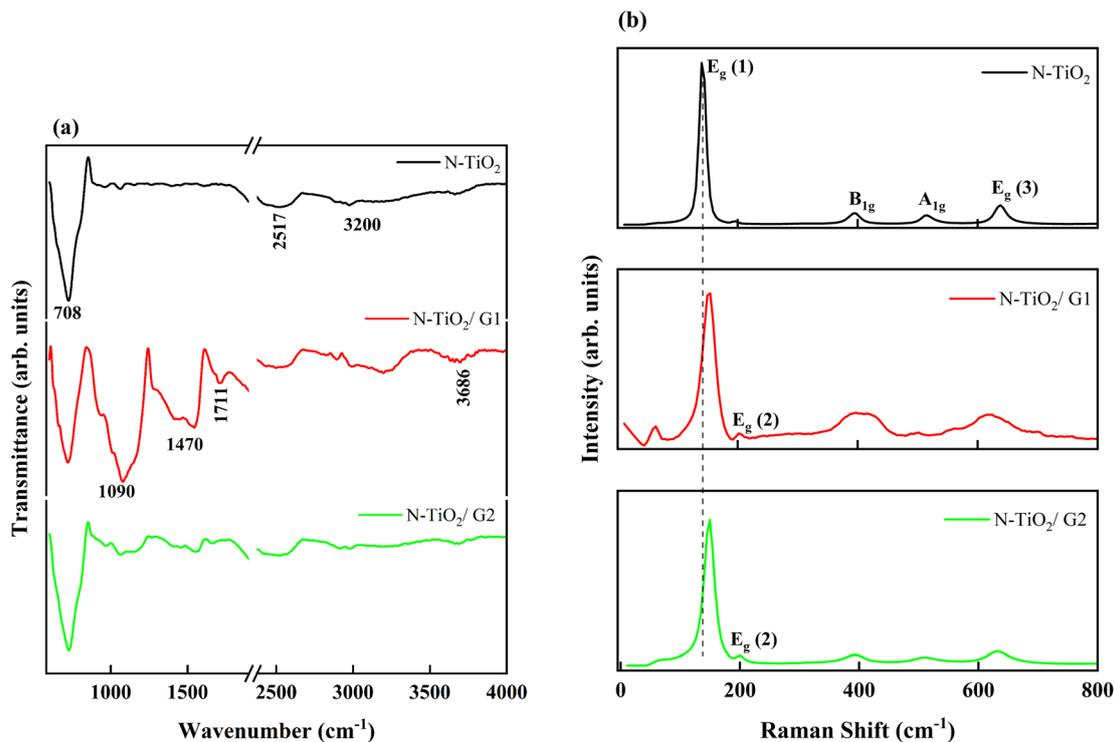
Fig. 5 (a) FTIR spectra of N-TiO<sub>2</sub> and graphene supported N-TiO<sub>2</sub>/G and Raman spectra of N-TiO<sub>2</sub> and graphene supported N-TiO<sub>2</sub>.
