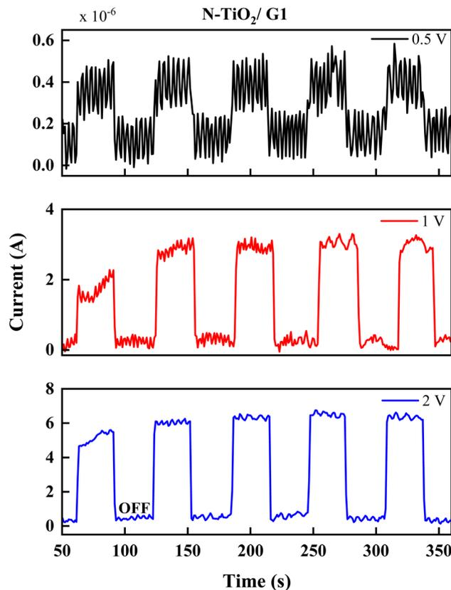
Fig. 12 The photodetection properties of a low concentration of graphene-supported N-TiO<sub>2</sub> at 0.5 V, 1 V and 2 V bias voltage.
