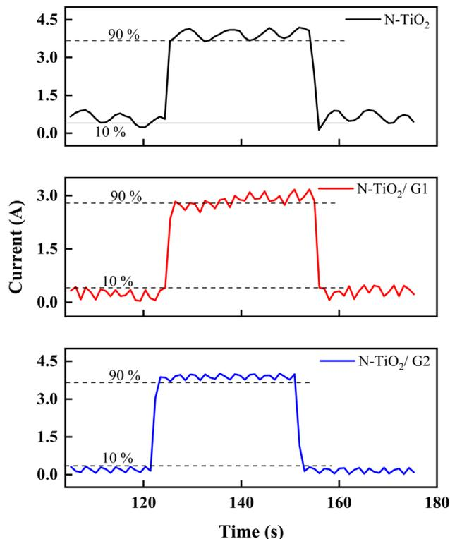
Fig. 14 The response characteristics of pristine and graphene-supported N-TiO<sub>2</sub> at 1 V bias voltage.
