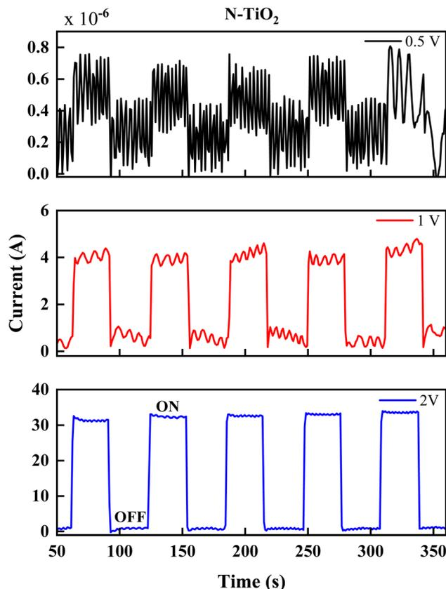
Fig. 11 The photodetection properties of pristine N-TiO<sub>2</sub> at 0.5 V, 1 V and 2 V bias voltage.
