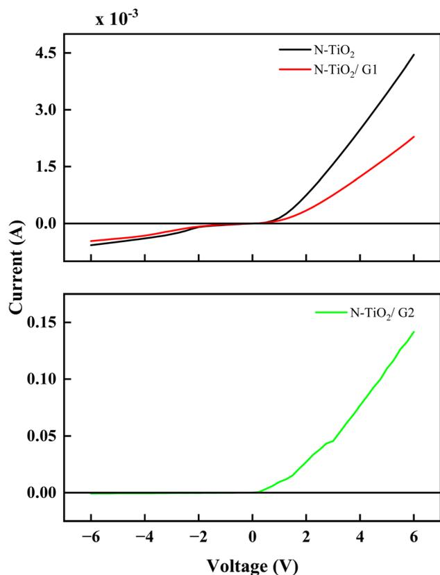
Fig. 9 The current–voltage characteristics of N-TiO<sub>2</sub> and graphene supported N-TiO<sub>2</sub>.
