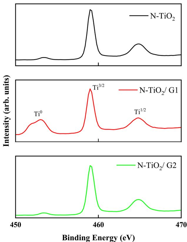
**Fig. 7** The Ti 2p core level XPS spectra for N-TiO<sub>2</sub> and graphene supported N-TiO<sub>2</sub>.
