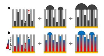
Fig. 1 Self-controlled growth of nanowires *via* thermal gradients. (a) Unstable growth of nanowires in template-assisted electrodeposition. (b) Suppression of growth instability by introducing temperature gradients across the nanoporous template, resulting in more uniform nanowire growth.
