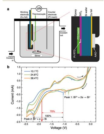
Fig. 2 (a) An electrodeposition cell capable of achieving local temperature gradients across nanoporous anodic aluminum oxide (AAO) template. (b) Cyclic voltammetry for bismuth under various bath temperatures. Red arrow indicates assigned overpotential, which is 70% between the two reduction peaks (peak 1 and 2).
