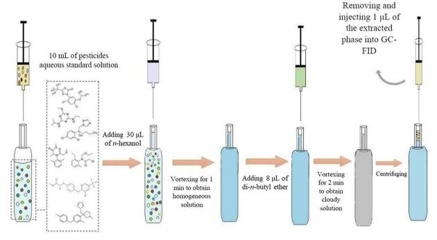
Fig. 1 Schematic of the extraction process
