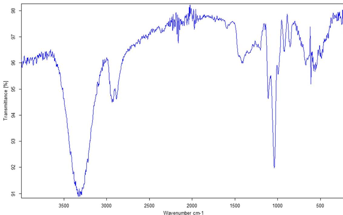
Fig. 7 FTIR spectrum obtained for SP2 on CaF<sub>2</sub> substrate.
