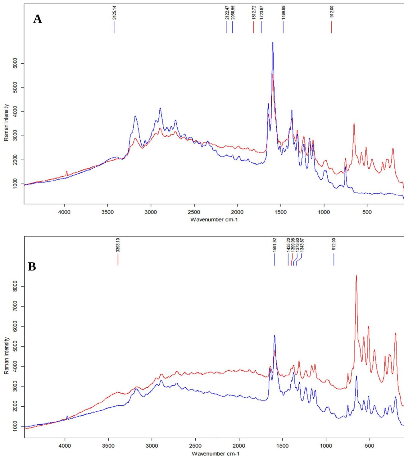
Fig. 6 (A) – Comparison of the substrate's influence on the Raman spectroscopy spectrum for SP1. Blue represents the spectrum for the steel plate, while red represents the spectrum for CaF<sub>2</sub>. (B) – Comparison of the effect of the UF process on the spectra of SP1 and SP2 on the CaF<sub>2</sub> substrate. Blue indicates SP1 (without UF), while red suggests SP2 (UF).
