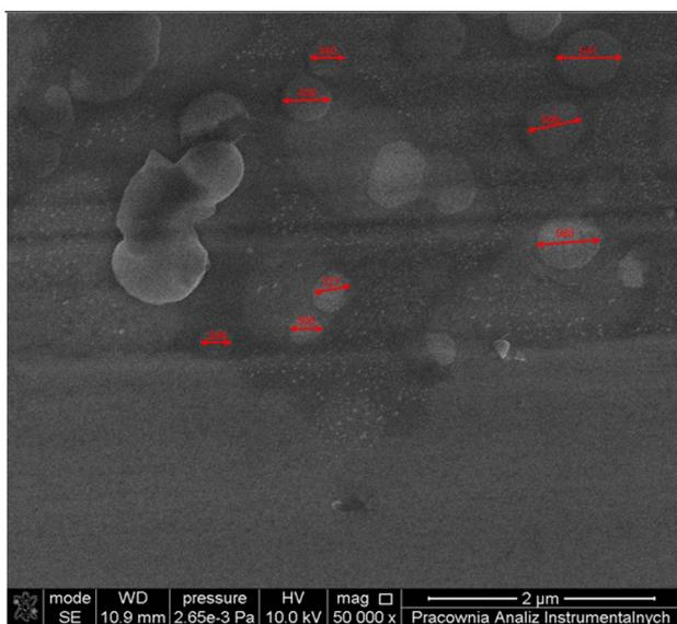
Fig. 4 HR-SEM image of CoPPIX nanoparticles for SP2.
