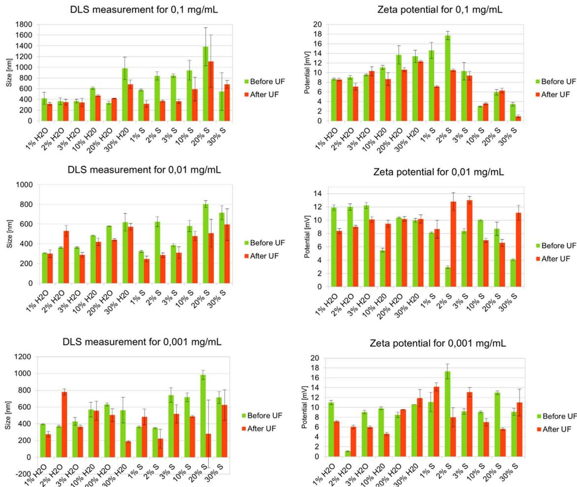
Fig. 2 Results of hydrodynamic size and zeta potential DLS measurements for Co(III)PPIX nanoparticles, where concentration of Co(III)PPIX at 0.1 mg mL<sup>-1</sup> (A), 0.01 mg mL<sup>-1</sup> (B) and 0.001 mg mL<sup>-1</sup> (C).
