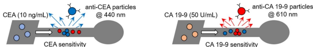
Scheme 8 \mu PAD for the quantification of colorectal cancer biomarkers, carcinoembryonic antigen (CEA) and carbohydrate antigen 19-9 (CA 19-9) in human blood and serum. 58
