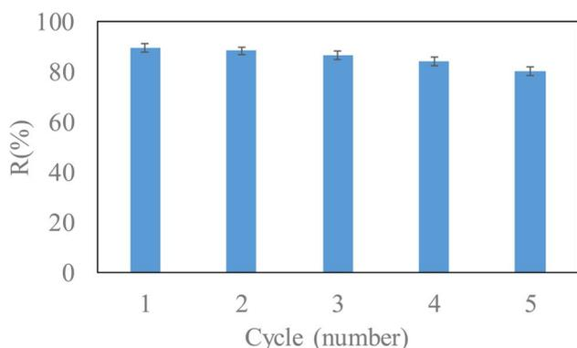
Fig. 12 The regeneration of PEG/MoS<sub>2</sub>@BC for Cr(vi) removal (reaction conditions: dosage of PEG/MoS<sub>2</sub>@BC, 0.1 g L<sup>-1</sup>; reaction time, 360 min; initial concentration of Cr(vi), 20 mg L<sup>-1</sup>; temperature, 318.15 K; solution pH, 6).
