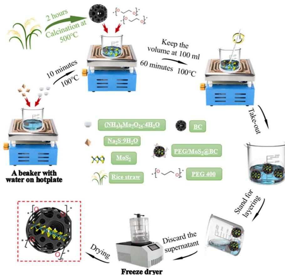
Fig. 1 The synthesis procedure for the PEG/MoS<sub>2</sub>@BC composite.
