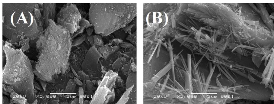
Fig. 2 SEM images of BC (A) and PEG/MoS<sub>2</sub>@BC (B).
