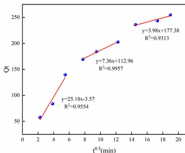
Fig. 7 The intraparticle diffusion model for Cr(vi) on PEG/MoS<sub>2</sub>@BC.
