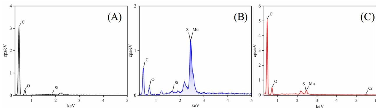
Fig. 3 EDS spectra of BC (A), PEG/MoS<sub>2</sub>@BC (B), and PEG/MoS<sub>2</sub>@BC-Cr (C).
