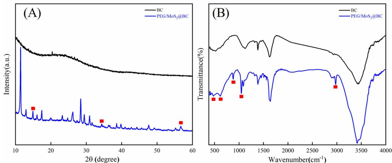
Fig. 4 XRD patterns (A) and FT-IR spectra (B) of biochar and PEG/MoS<sub>2</sub>@BC.
