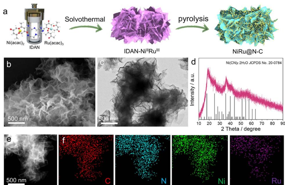
Fig. 1 (a) Schematic demonstration for synthesis of Ni<sub>5</sub>Ru@N-C; (b) SEM image, (c) TEM image, (d) XRD pattern (e) STEM image and (f) corresponding EDX element mappings of IDAN-Ni<sup>2+</sup>/Ru<sup>3+</sup> OCP.
