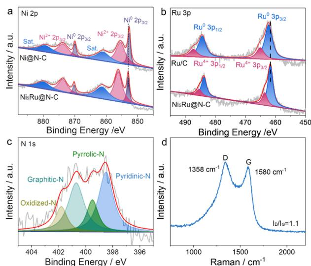
Fig. 3 (a) Ni 2p XPS spectra of Ni<sub>5</sub>Ru@N-C and Ni@N-C; (b) Ru 3p XPS spectra Ni<sub>5</sub>Ru@N-C and commercial Ru/C; (c) N 1s XPS spectra and (d) Raman spectrum of Ni<sub>5</sub>Ru@N-C.
