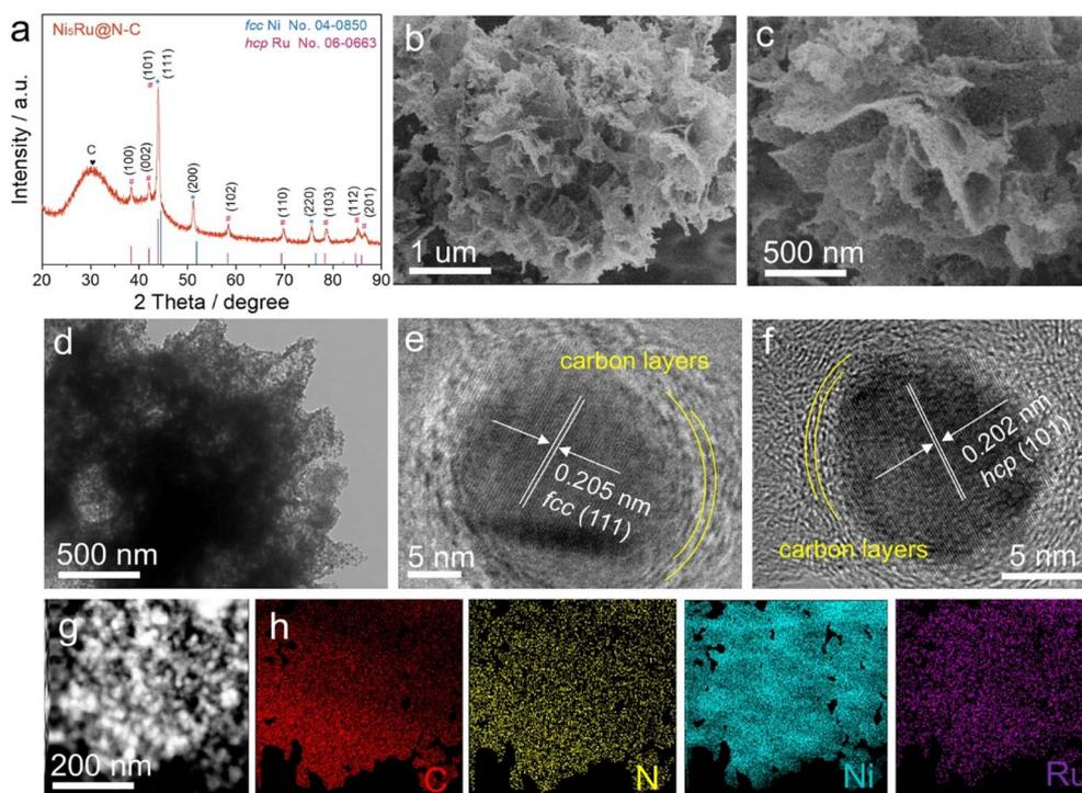
Fig. 2 (a) XRD pattern, (b and c) SEM images; (d) TEM image, (e and f) HRTEM images, (g) STEM image and (h) corresponding EDX element mappings of Ni<sub>5</sub>Ru@N-C.
