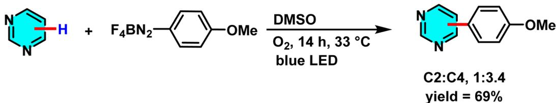
Scheme 91 Photocatalyst-free, visible-light-induced C–H arylation of pyrimidine using aryl diazonium salts.
