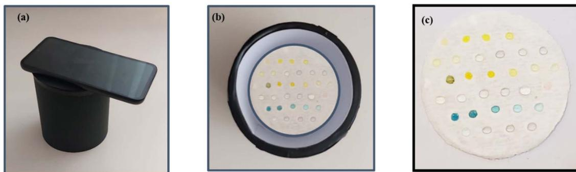
**Scheme 3** Cylindrical box format designed for capturing digital images: (a) a handmade box with an A54 smartphone placed on top, fixed at a height of 110 cm; (b) the bottom part of the box with the microarray test fixed for image acquisition, (c) microarray paper that contains the colored product, with concentrations ranging from  $1 \text{ ng ml}^{-1}$  to  $1 \mu\text{g ml}^{-1}$ .
