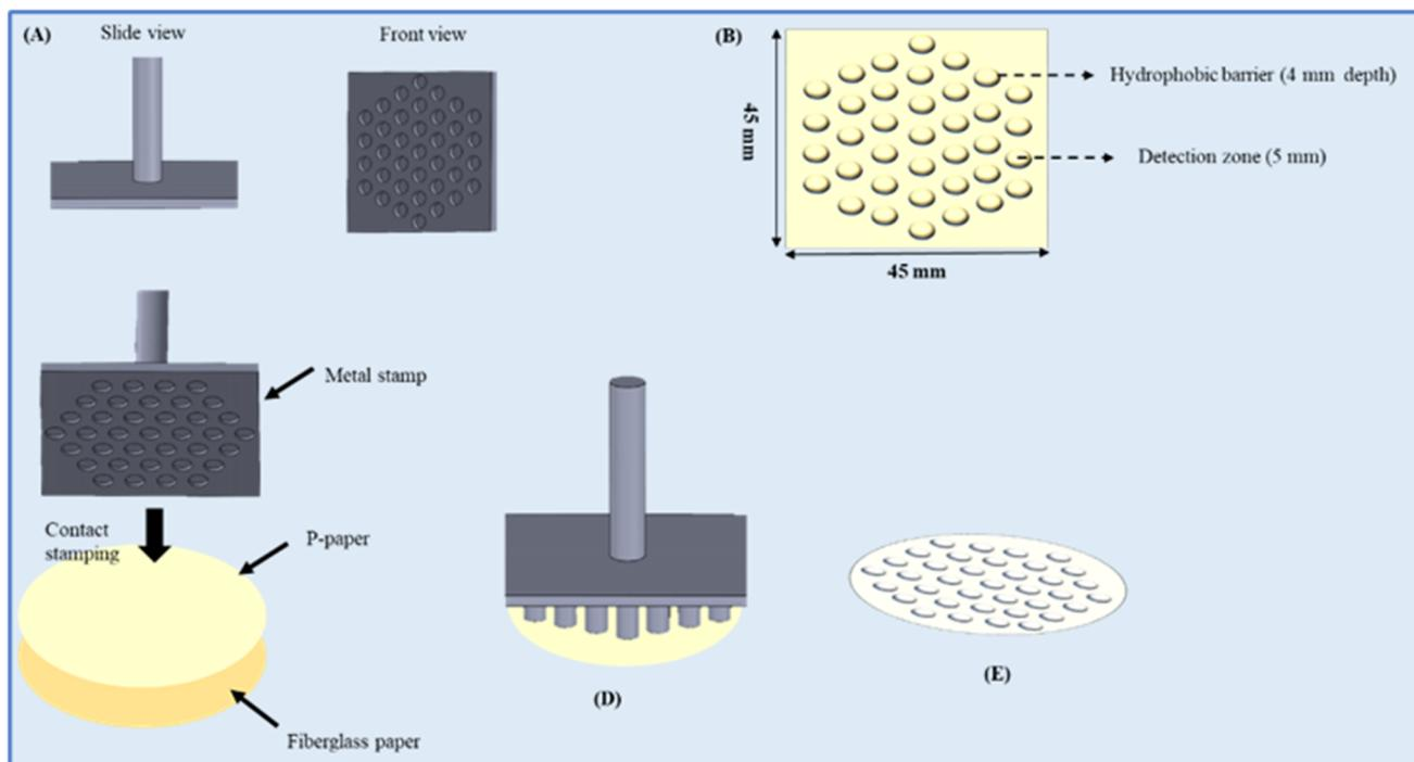
**Scheme 2** Fabrication steps for the microarray PCS by contact stamping. (A) Photograph of the custom-designed stamping device, (B) stamping pattern of the hydrophobic barrier and semi-hydrophobic detection zone, (C) a paraffinized paper (p-paper) is placed over the native fiberglass paper (n-paper) surface, (D) the metal stamp is heated to 180 °C and pressed into contact for 20 seconds, (E) represents a typical microarray PCS fabricated by the proposed method.
