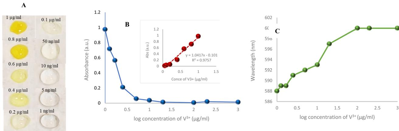
Fig. 6 Colorimetric results for  $\text{V}^{3+}$  determination using DES-PCD. (A) Images for the PCD displayed different  $\text{V}^{3+}$  amounts. (B) The calibration curve indicated the correlation between the value of RGB-based absorbance and the concentration of  $\text{V}^{3+}$ . (C) The correlation between wavelength and the log concentration of  $\text{V}^{3+}$ .
