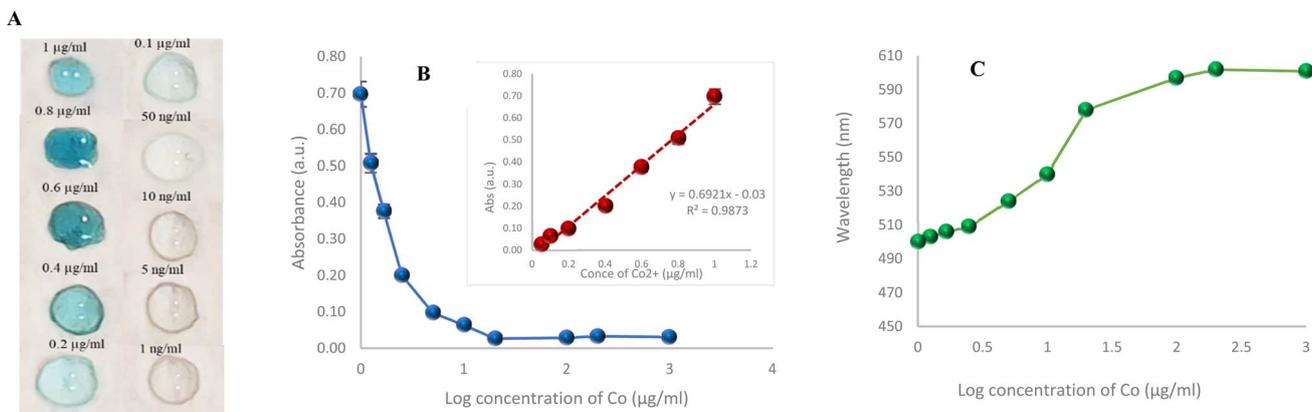
Fig. 7 Colorimetric results for  $\text{Co}^{2+}$  determination using DES-PCS. (A) Images for the PCS displayed different  $\text{Co}^{2+}$  amounts. (B) The calibration curve indicated the correlation between the value of RGB-based absorbance and the concentration of  $\text{Co}^{2+}$ . (C) The correlation between wavelength and the log concentration of  $\text{Co}^{2+}$ .
