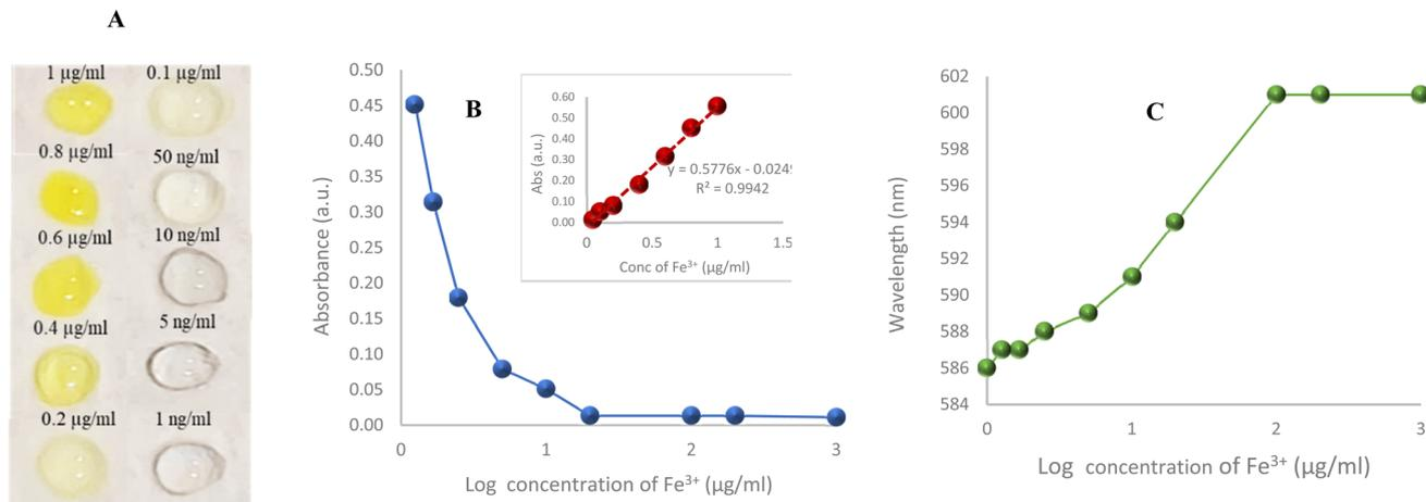
Fig. 5 Colorimetric results for  $\text{Fe}^{3+}$  determination using DES-PCS. (A) Images for the PCS displayed different  $\text{Fe}^{3+}$  amounts. (B) The calibration curve indicated the correlation between the value of RGB-based absorbance and the concentration of  $\text{Fe}^{3+}$ . (C) The correlation between wavelength and the log concentration of  $\text{Fe}^{3+}$ .
