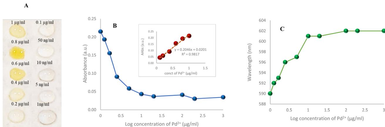
**Fig. 8** Colorimetric results for Pd<sup>2+</sup> determination using DES-PCS. (A) Images for the PCS displayed different Co<sup>2+</sup> amounts. (B) The calibration curve indicated the correlation between the value of RGB-based absorbance and the concentration of Pd<sup>2+</sup>. (C) The correlation between wavelength and the log concentration of Pd<sup>2+</sup>.
