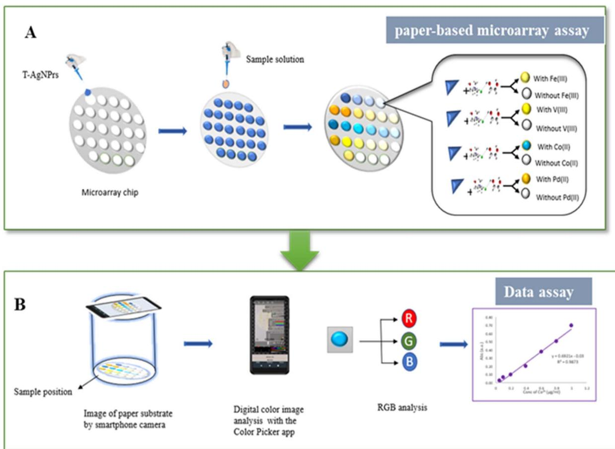
**Scheme 4** (A) Illustration of the colorimetric paper-based microarrays fabricated on fiberglass for the simultaneous detection of multiple metal ions ( $\text{Fe(III)}$ ,  $\text{V(III)}$ ,  $\text{Co(II)}$ , and  $\text{Pd(II)}$ ). (B) The design of a smartphone-based portable reader with an app to acquire colorimetric changes from the microarray and report the results.
