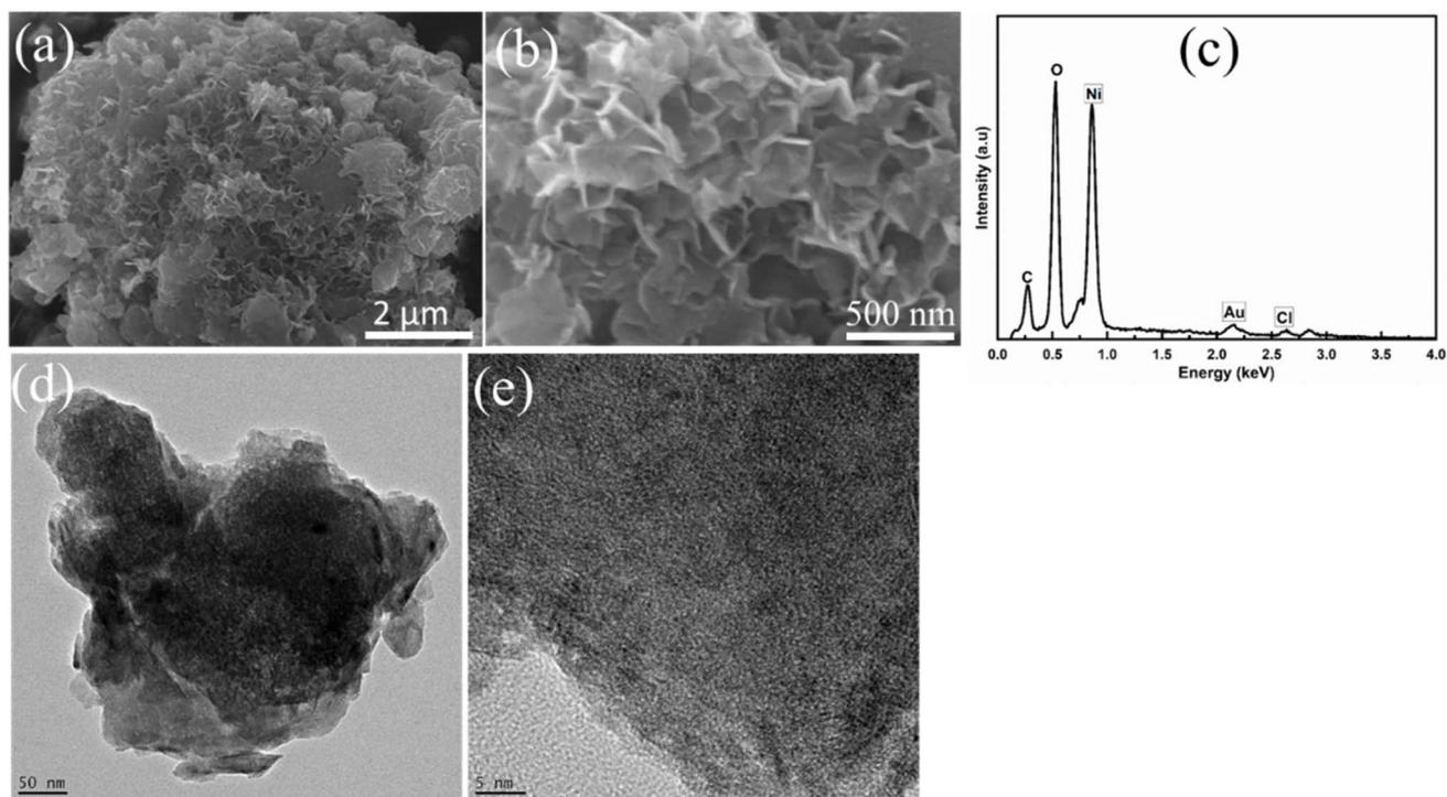
Fig. 2 (a) FESEM image of the as-prepared anodic  $\text{Ni}(\text{OH})_2$  showing the formation of nanoflowers, (b) high-magnification image of a single nanoflower, (c) EDX spectrum showing the composition of  $\text{Ni}(\text{OH})_2$  nanoflowers, (d) low-resolution TEM image, and (e) HRTEM image of the  $\text{Ni}(\text{OH})_2$  nanoflowers.
