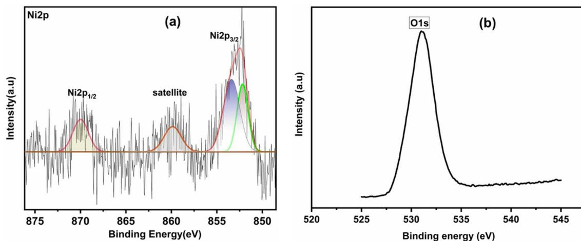
Fig. 6 High-scan XPS spectrum of (a) Ni 2p and (b) oxygen O 1s of the NiO NPs prepared via anodization in a 1 M aqueous NaCl electrolyte.
