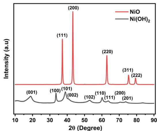
Fig. 1 XRD pattern of the Ni(OH)<sub>2</sub> nanoflowers and NiO NPs prepared via anodization in 1 M aqueous NaCl electrolyte.
