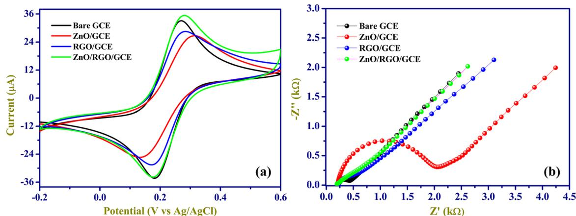
Fig. 5 CVs (a) and EIS (b) of bare GCE (black), ZnO/GCE (red), RGO/GCE (blue), and ZnO/RGO/GCE (green) in 0.1 M KCl containing 2 mM  $[\text{Fe}(\text{CN})_6]^{3-/4-}$  (inset: Randles equivalent circuit).
