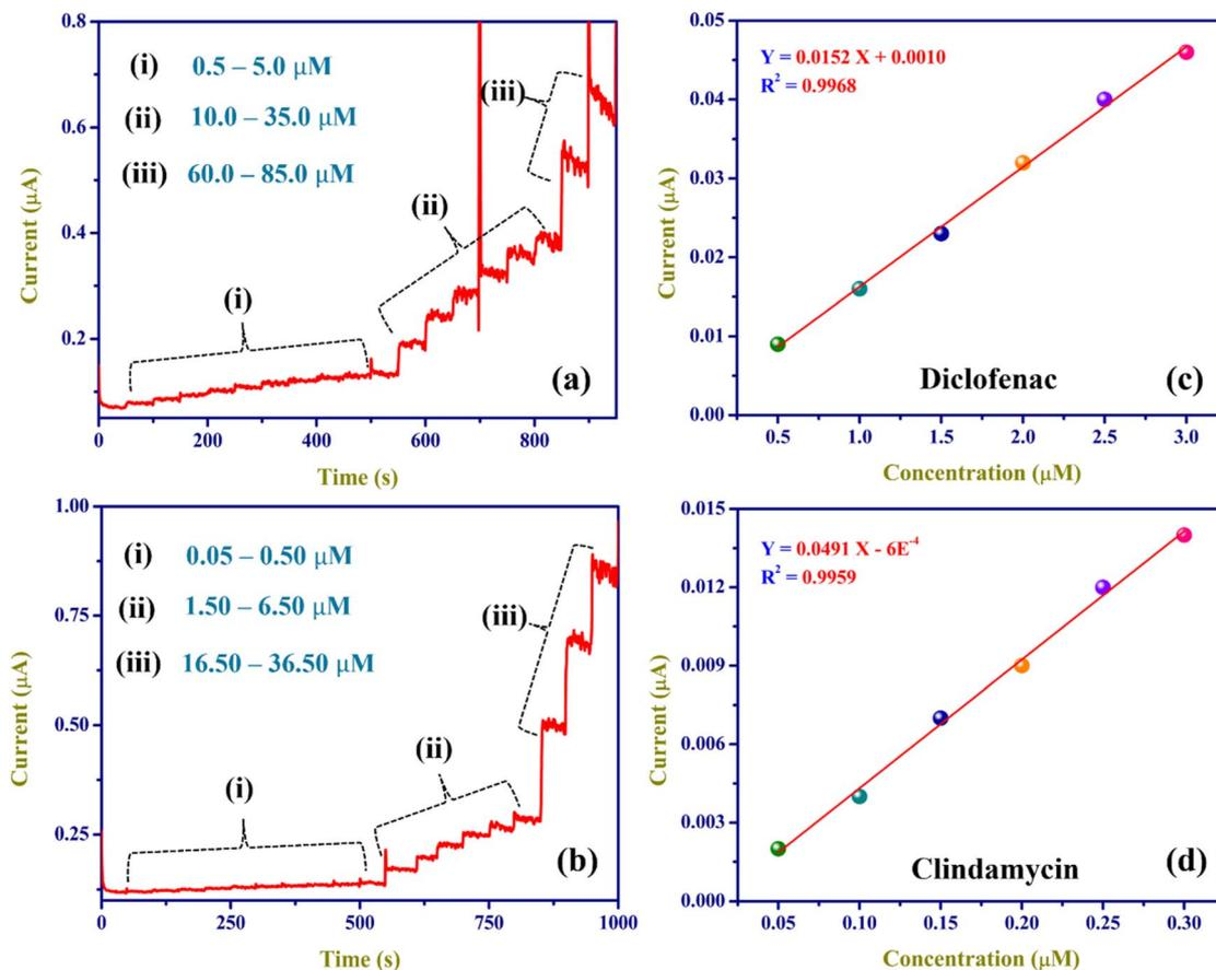
Fig. 9 Amperograms were recorded using ZnO/RGO/GCE with DCF at 0.56 V and CMC at 0.8 V, ranging from 0.5 to 85.0  $\mu\text{M}$  (a) and from 0.05 to 36.50  $\mu\text{M}$  (b) at 750 rpm (0.1 M PBS, pH 7.4), respectively. The linear calibration curves were made for a concentration of DCF (0.5 to 85.0  $\mu\text{M}$ ) (c) and CMC (0.05 to 36.50  $\mu\text{M}$ ) (d) vs. oxidation current ( $\mu\text{A}$ ).
