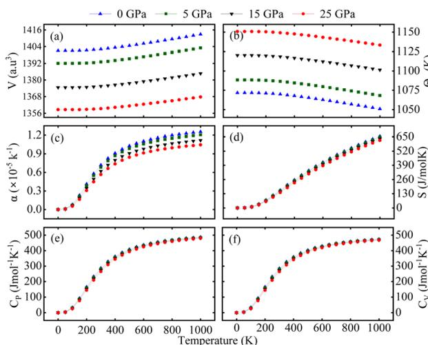
Fig. 5 Computed (a) volume ( $V$ ), (b) Debye temperature ( $\theta_D$ ), (c) absorption coefficient ( $\alpha$ ), (d) entropy ( $S$ ), and (e) and (f) specific heat capacity at constant pressure/constant ( $C_P/C_V$ ) volume of the  $\text{Lu}_2\text{-CoCrO}_6$  structure.
