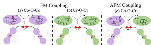
Fig. 7 Schematic illustration of the ferromagnetic (FM) superexchange interactions of (a and b) Co–O–Co/Cr–O–Cr and (c) antiferromagnetic (AFM) coupling between  $\text{Co}^{3+}\text{-}3d^6$  and  $\text{Cr}^{3+}\text{-}3d^3$  ions *via* oxygen in the  $\text{Lu}_2\text{CoCrO}_6$  structure.
