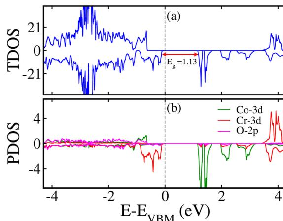
Fig. 8 Calculated spin-polarized (a) total density of states (TDOS) and (b) partial density of states (PDOS), highlighting the role of Co-3d/Cr-3d/O-2p orbitals around the Fermi level for the  $\text{Lu}_2\text{CoCrO}_6$  structure.
