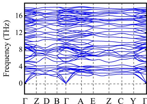
Fig. 3 Calculated phonon spectrum of the  $\text{Lu}_2\text{CoCrO}_6$  structure.
