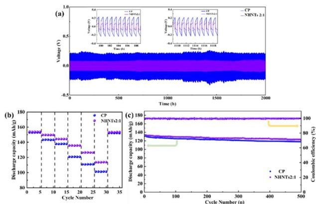
Fig. 4 (a) Voltage versus time plots symmetric cell under a current density of 0.1 mA cm<sup>-2</sup>; (b) C-rate capability; (c) cycling performance at 1C.
