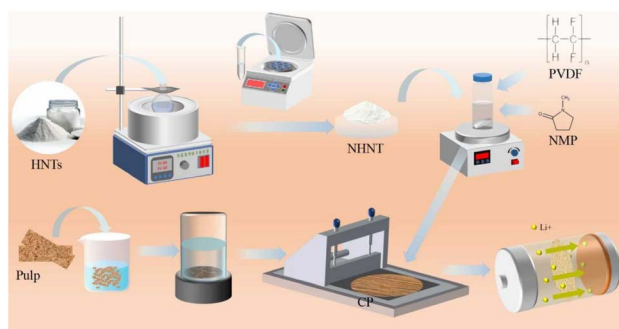
Scheme 1 Schematic diagram of preparation process for the separator.
