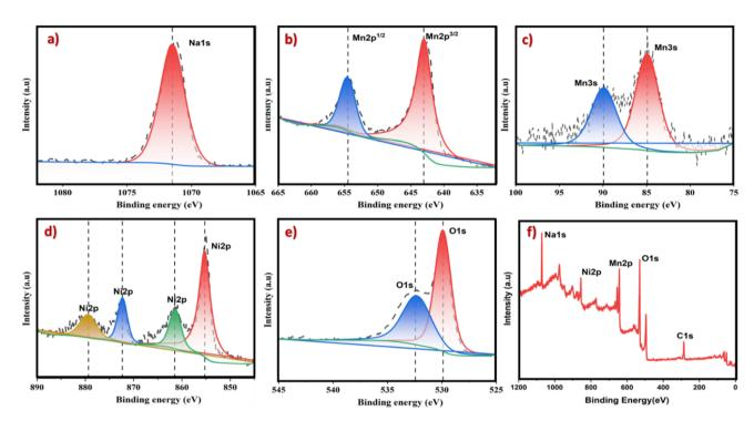
Fig. 4 X-ray photoelectron spectroscopy (XPS) analysis of Na<sub>0.67</sub>Ni<sub>0.33</sub>O<sub>2</sub>: (a) Na 1s spectrum, (b) Mn 2p spectrum, (c) Mn 3 s spectrum, (d) Ni 2p spectrum, (e) O 1s spectrum, and (f) survey spectrum.
