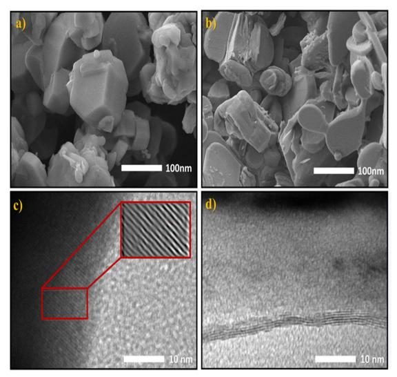
Fig. 3 SEM (a  $\vartheta$  b) and TEM (c  $\vartheta$  d) images of Na<sub>0.67</sub>Mn<sub>0.67</sub>Ni<sub>0.33</sub>O<sub>2</sub> synthesised through solid state reaction technique.
