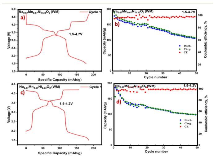
Fig. 6 Electrochemical performance of wet-milled (WM) Na<sub>0.67</sub>Mn<sub>0.67</sub>Ni<sub>0.33</sub>O<sub>2</sub> electrodes: (a) initial charge-discharge profiles in the voltage range 1.5-4.7 V, (b) cycling stability at 1.5-4.7 V, (c & d) 1.5-4.2 V.
