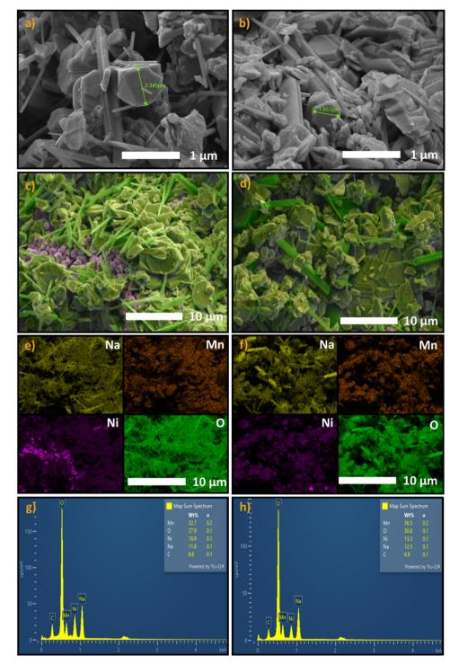
Fig. 7 SEM micrographs, elemental distribution maps, and EDS spectra of  $Na_{0.67}Mn_{0.67}Ni_{0.33}O_2$  synthesized *via* dry milling (a, c, e and g) and wet milling (b, d, f and h).
