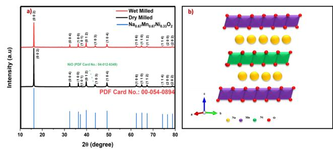
Structural characterization of Na<sub>0.67</sub>Mn<sub>0.67</sub>Ni<sub>0.33</sub>O<sub>2</sub> (a) XRD pattern. (b) P2-type crystal structure schematic.
