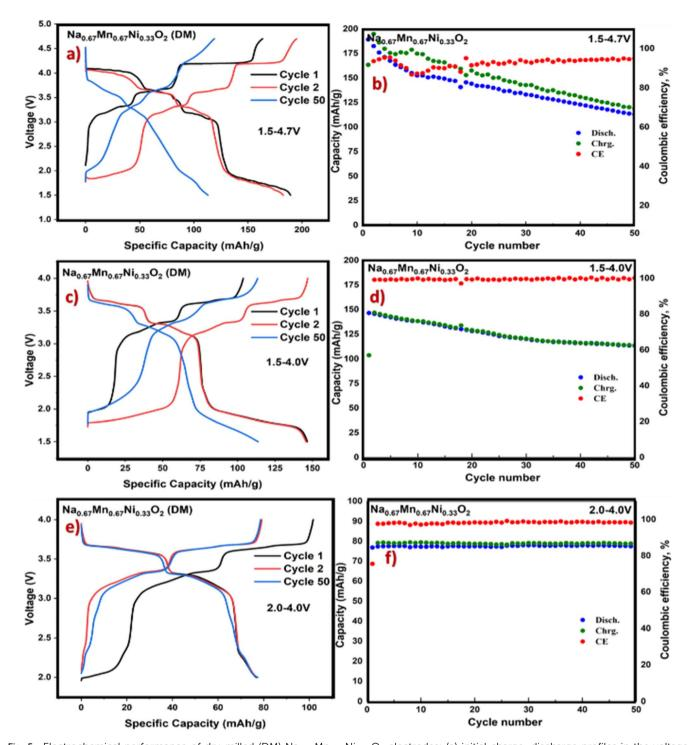
Fig. 5 Electrochemical performance of dry-milled (DM)  $Na_{0.67}Nn_{0.67}Ni_{0.33}O_2$  electrodes: (a) initial charge-discharge profiles in the voltage range 1.5-4.7 V, (b) cycling stability at 1.5-4.7 V, (c & d) 1.5-4.0 V and (e & f) 2.0-4.0 V.
