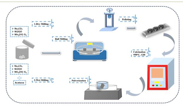
Fig. 1 Methodology for the synthesis of Na<sub>0.67</sub>Mn<sub>0.67</sub>Ni<sub>0.33</sub>O<sub>2</sub>.
