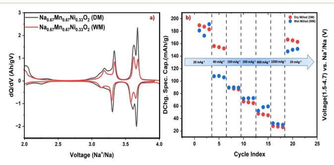
Fig. 8 (a) Differential capacity (dQ/dV) curves of  $Na_{0.67}Mn_{0.67}Ni_{0.33}O_2$  electrodes synthesized by dry milling (DM) and wet milling (WM), (b) Rate capability of the dry-milled (DM) and wet milled (WM)  $Na_{0.67}Mn_{0.67}Ni_{0.33}O_2$  electrode at various current densities.
