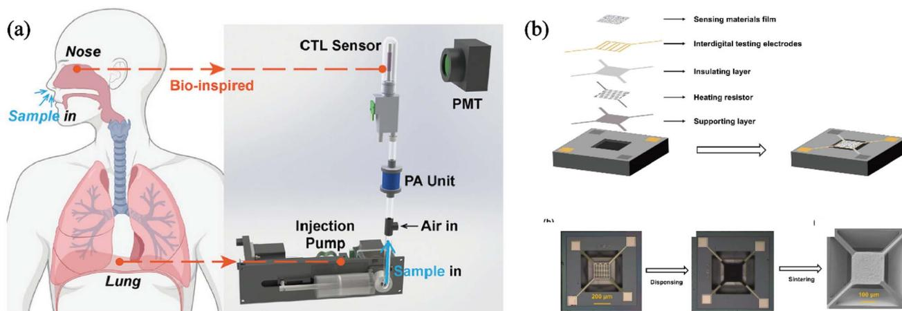
Fig. 3 (a) Sensor array used as an electronic nose. Reproduced with permission.<sup>28</sup> Copyright from Wiley, 2024. (b) Schematic of a common MOS framework. Reproduced with permission.<sup>29</sup> Copyright from MDPI, 2025.
