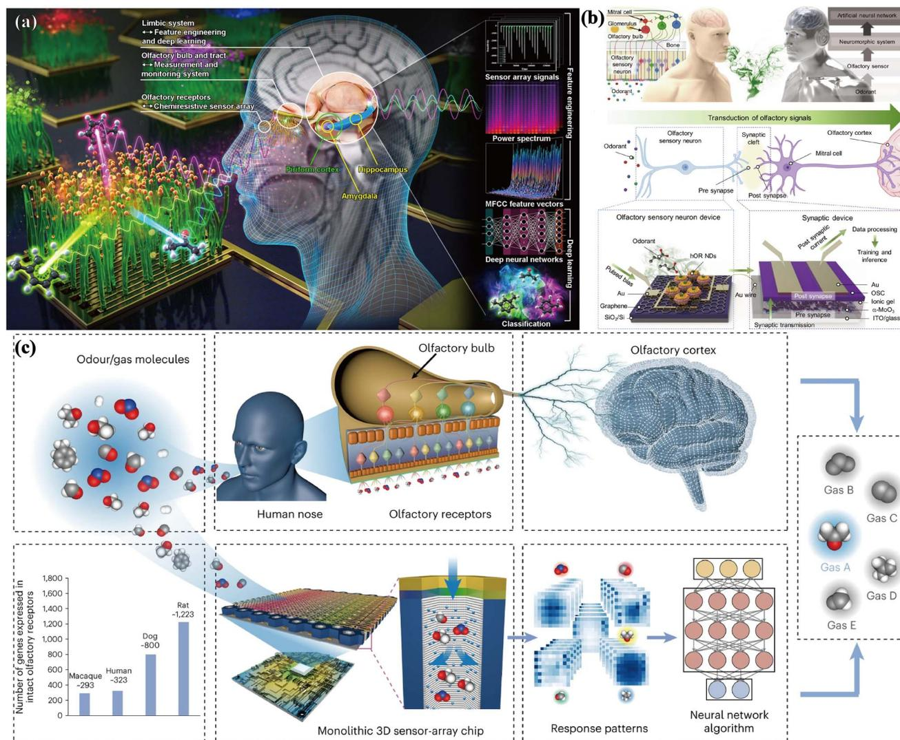
Fig. 1 Schematic of the pathway of the biomimetic olfactory system. (a) Reproduced with permission.<sup>7</sup> Copyright from Springer Nature, 2024. (b) Reproduced with permission.<sup>8</sup> Copyright from AAAS, 2024. (c) Reproduced with permission.<sup>9</sup> Copyright from Springer Nature, 2024.
