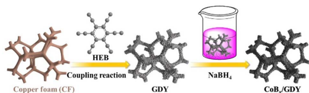
Scheme 1 The synthesis of \text{CoB}_x nanosheets grown in situ on GDY nanowalls at room temperature.
