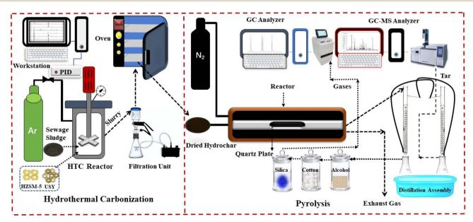
Fig. 1 Schematic diagram of integrated HTC-Py setup.
