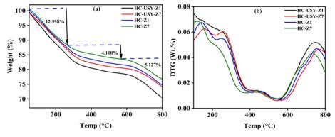
Fig. 10 Thermal analysis; (a) TGA of HC-Z1, HC-Z7, HC-USY-Z1, HC-USY-Z7 and (b) DTG of HC-Z1, HC-Z7, HC-USY-Z1, HC-USY-Z7.
