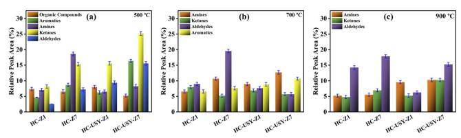
Fig. 12 Effects of various temperatures on tar composition of all catalyzed HC; HC-Z1, HC-Z7, HC-USY-Z1, HC-USY-Z7 (a) 500 °C, (b) 700 °C, (c) 900 °C.
