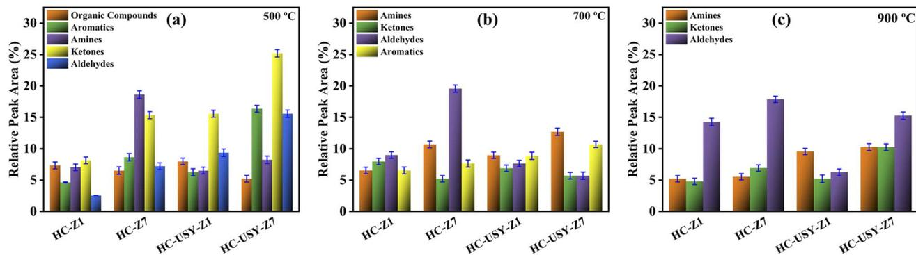
Fig. 12 Effects of various temperatures on tar composition of all catalyzed HC; HC-Z1, HC-Z7, HC-USY-Z1, HC-USY-Z7 (a) 500 °C, (b) 700 °C, (c) 900 °C.
