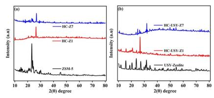
Fig. 8 XRD of catalysts and catalyzed HC; (a) HZSM-5, HC-Z1, HC-Z7 (b) USY-zeolite, HC-USY-Z1, HC-USY-Z7.
