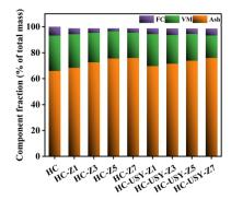
Fig. 2 Component fraction of HC with increasing percentages of zeolite catalyst.
