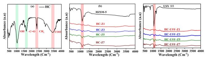
Fig. 6 FTIR spectrum of (a) uncatalyzed HC, catalyst, and catalyzed HC with different catalysts loading (b) HZSM-5, HC-Z1 to HCZ7, (c) USY-zeolite, HC-USY-Z1 to HC-USY-Z7.
