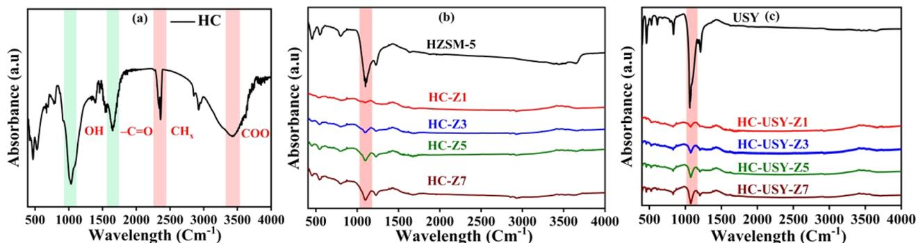
Fig. 6 FTIR spectrum of (a) uncatalyzed HC, catalyst, and catalyzed HC with different catalysts loading (b) HZSM-5, HC-Z1 to HC-Z7, (c) USY zeolite, HC-USY-Z1 to HC-USY-Z7.
