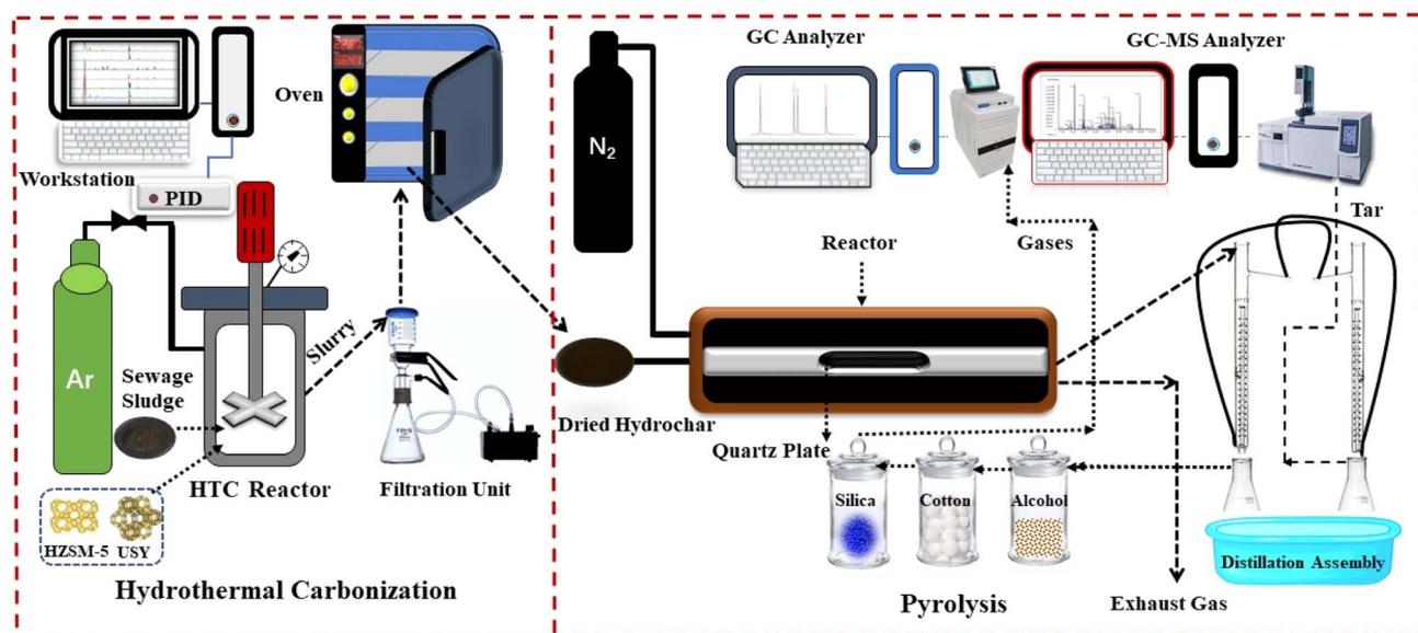
Fig. 1 Schematic diagram of integrated HTC-Py setup.
