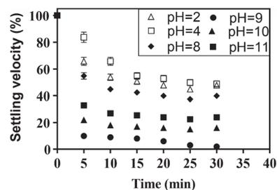
Fig. 21 Effect on settling velocity of magnetic nanoparticles grafted on hyperbranched polyglycerol, demonstrating their pH-responsive colloidal stability and aggregation behavior in aqueous media. Adapted from ref. 209 with permission from Elsevier, copyright 2020.
