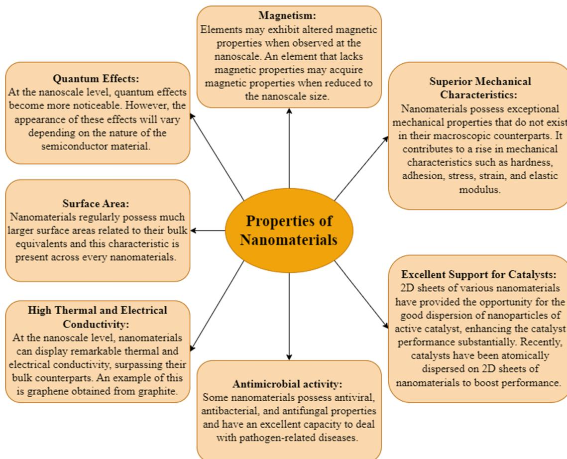
Fig. 9 Exploring the characteristics of materials at the nanoscale.<sup>76,91,92</sup>
