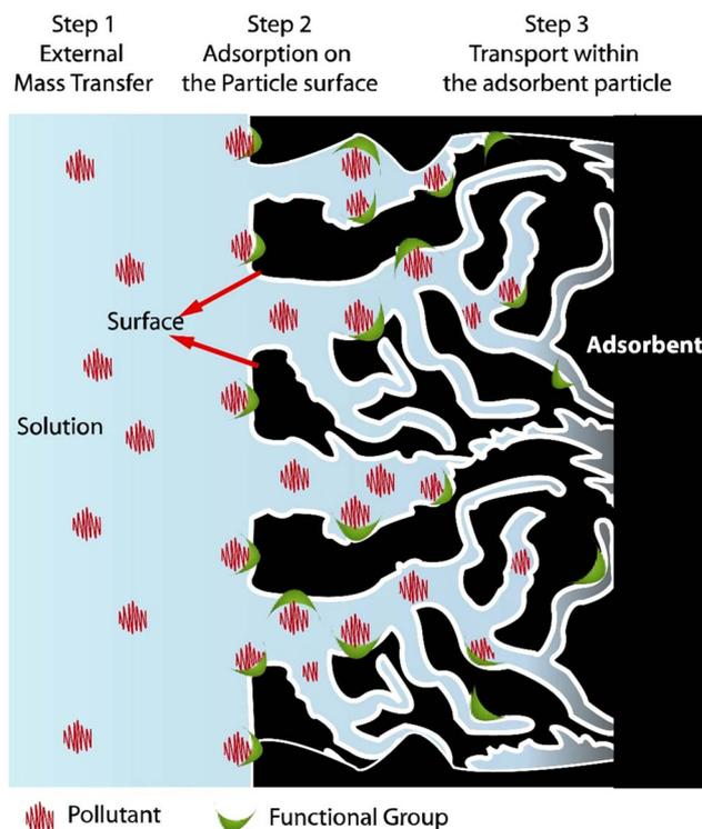
Fig. 5 Schematic illustration of the adsorption technique and its mechanics. Adapted from ref. 57 with permission from Elsevier, copyright 2024.
