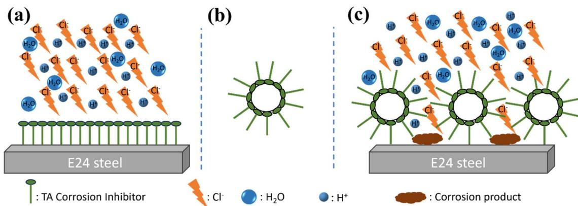
Fig. 13 Representative scheme: (a) metal protection at low TA inhibitor concentrations, (b) congestion of the TA inhibitor molecule at high concentrations, and (c) attack of the steel surface by chlorides at concentrations that exceed the critical level.
