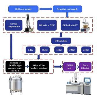
Fig. 1 Schematic flowchart of the experimental procedure.
