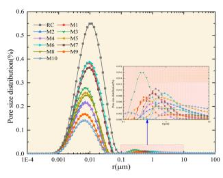
Fig. 4 Average pore size distribution of water-saturated coal samples under varied temperature and time conditions.
