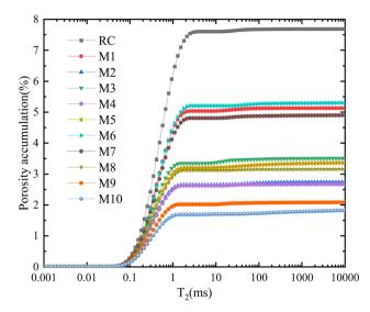
Fig. 6 Cumulative porosity of coal samples under various temperature and time conditions.
