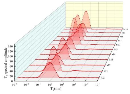
$T_2$  distribution curves of water-saturated coal samples under varied temperature and time conditions.
