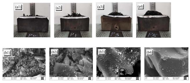
Fig. 8 (a) Optical images (a1-a4) and (b) SEM images (b1-b4) of residual chars from combustion of P0, P1, P3, and P5.
