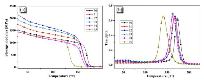
(a) E' and (b)  $\tan \delta$  versus temperature curves of epoxy thermosets
