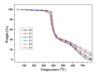
Fig. 5 TGA curves of epoxy thermosets in air.
