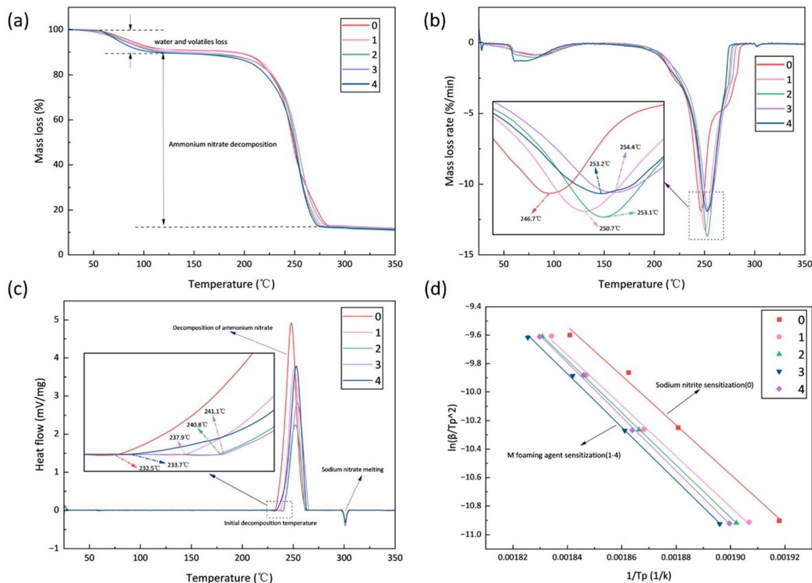
Fig. 7 (a) TG; (b) DTG curves of the explosive samples at a heating rate of 5 K min<sup>-1</sup>; (c) DSC curves of the explosive samples at a heating rate of 5 K min<sup>-1</sup>; (d) Kinetic parameter curves obtained by Kissinger fitting based on the peak temperatures of the DSC curves.
