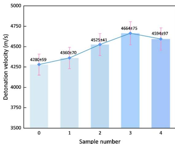
Fig. 5 Detonation velocity of the explosive samples.
