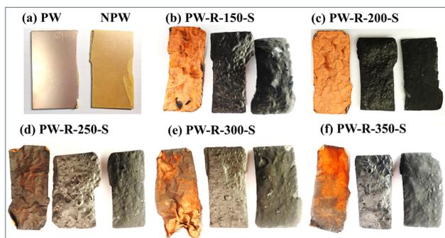
Fig. 12 (a) The metallic and non-metallic surfaces of PL-WCCL; the metallic and non-metallic parts of PL-WCCL obtained through rotary furnace heat treatment at different temperatures: (b) 150 °C, (c) 200 °C, (d) 250 °C, (e) 300 °C, (f) 350 °C.
