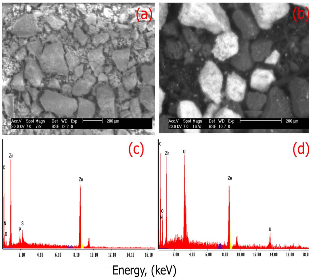
Fig. 3 SEM images of (a) PMA@ZIF-8 and (b) PMA@ZIF-8 loaded with U(vi). EDX analyses of (c) PMA@ZIF-8 and (d) PMA@ZIF-8 loaded with U(vi).
