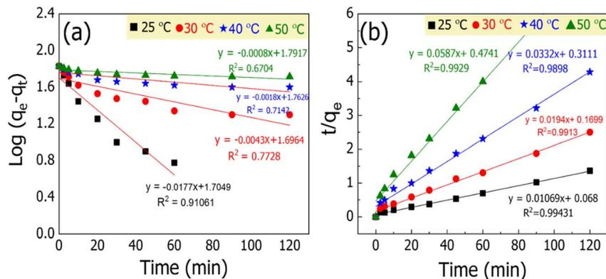
Fig. 9 Experimental and linear kinetic models for the adsorption of U(vi) onto the PMA@ZIF-8 composite: (a) pseudo-first-order and (b) pseudo-second-order models.
