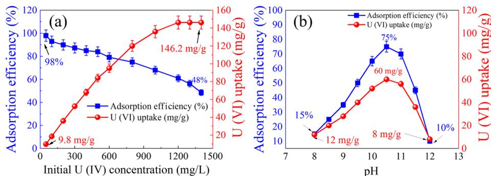
Fig. 6 Effect of (a) initial concentration and (b) solution pH on the removal percentage and U(vi) uptake by the PMA@ZIF-8 composite from alkaline aqueous solution.
