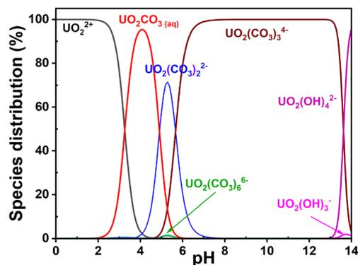
Fig. 7 The distribution of U(vi) species as a function of pH in the aqueous solution (400 mg L<sup>-1</sup> (0.0016804 M) uranium ions, 80 g L<sup>-1</sup> carbonate + 20 g bicarbonate).
