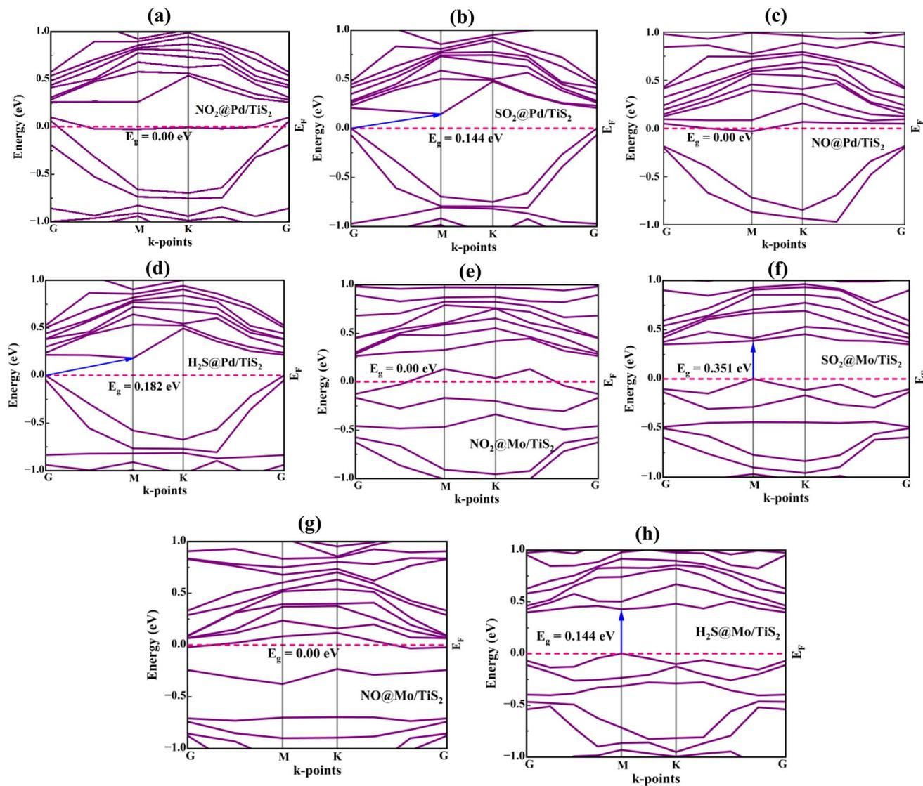
Fig. 7 Electronic band structures (a)  $\text{NO}_2$ @Pd/TiS<sub>2</sub>, (b)  $\text{SO}_2$ @Pd/TiS<sub>2</sub>, (c)  $\text{NO}$ @Pd/TiS<sub>2</sub>, and (d)  $\text{H}_2\text{S}$ @Pd/TiS<sub>2</sub>, (e)  $\text{NO}_2$ @Mo/TiS<sub>2</sub>, (f)  $\text{SO}_2$ @Mo/TiS<sub>2</sub>, (g)  $\text{NO}$ @Mo/TiS<sub>2</sub>, and (h)  $\text{H}_2\text{S}$ @Mo/TiS<sub>2</sub>.
