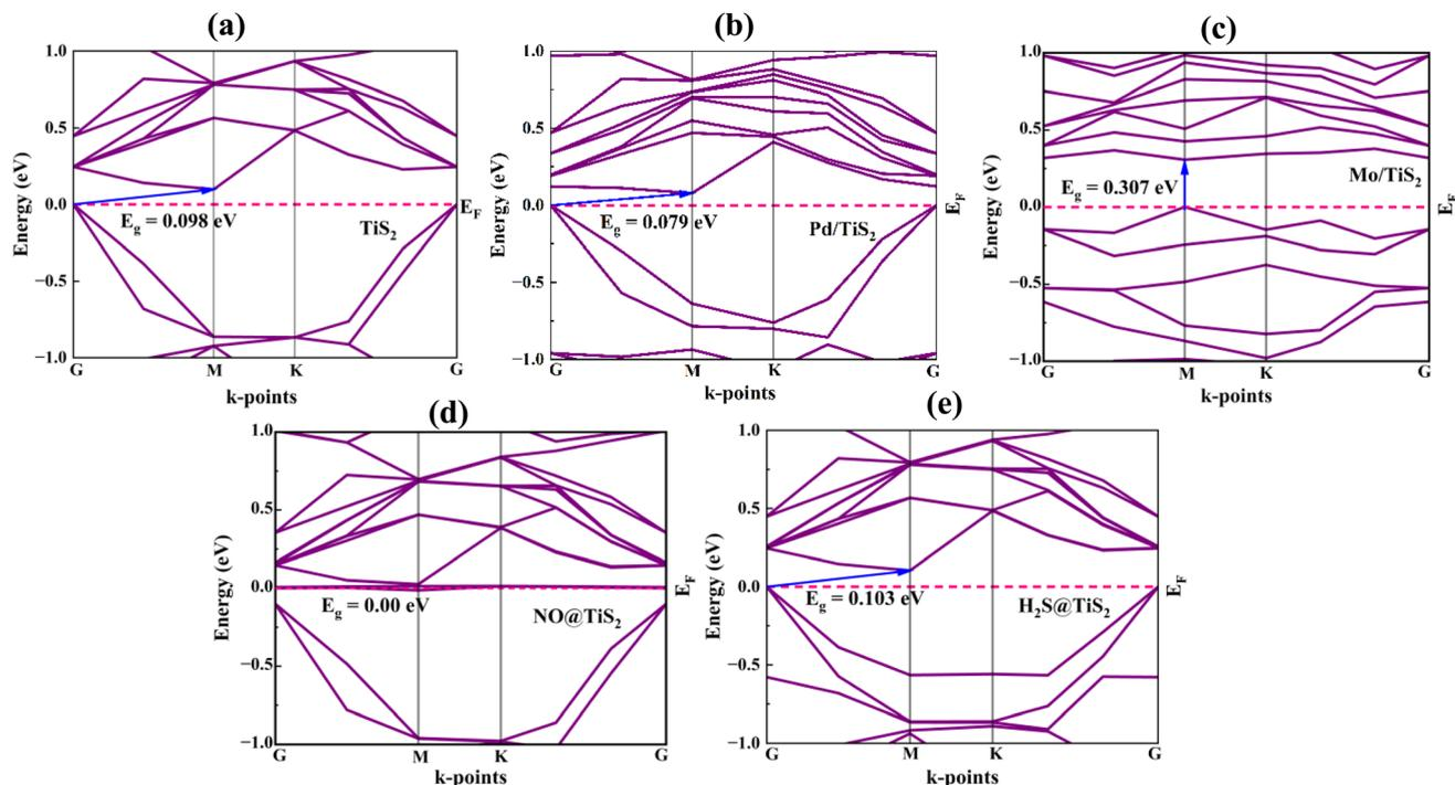
Fig. 6 Electronic band structures (a) pristine  $\text{TiS}_2$ , (b)  $\text{Pd}/\text{TiS}_2$ , (c)  $\text{Mo}/\text{TiS}_2$ , (d)  $\text{NO}@/\text{TiS}_2$ , and (e)  $\text{H}_2\text{S}@/\text{TiS}_2$ .
