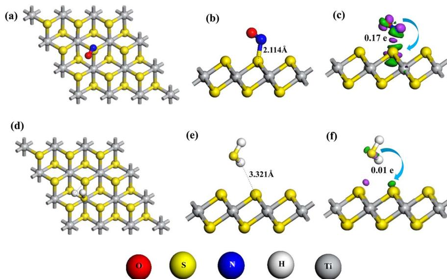
Fig. 3 Most stable optimized systems of adsorbed gas molecules on  $\text{TiS}_2$  monolayer: (a and b) top and side views of  $\text{NO@TiS}_2$ ; (d and e) top and side views of  $\text{H}_2\text{S@TiS}_2$ ; and (c and f) the corresponding charge density difference (CDD) of  $\text{NO@TiS}_2$  and  $\text{H}_2\text{S@TiS}_2$ .
