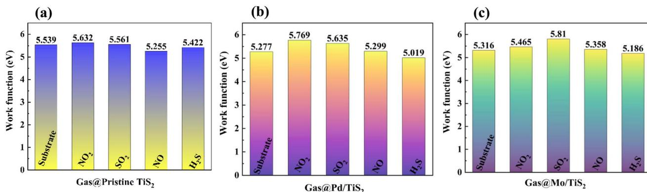
Fig. 10 Work function comparison for (a) pristine TiS<sub>2</sub>, (b) Pd/TiS<sub>2</sub>, (c) Mo/TiS<sub>2</sub> to different gases.
