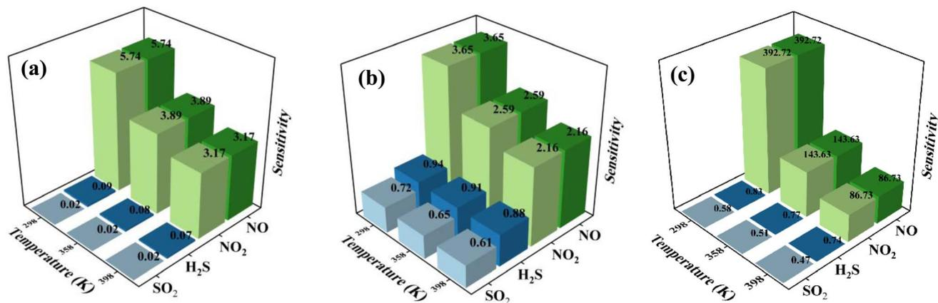
Fig. 9 Sensitivity of gas molecules on adsorption systems, (a) pristine TiS<sub>2</sub>, (b) Pd/TiS<sub>2</sub>, (c) Mo/TiS<sub>2</sub>.
