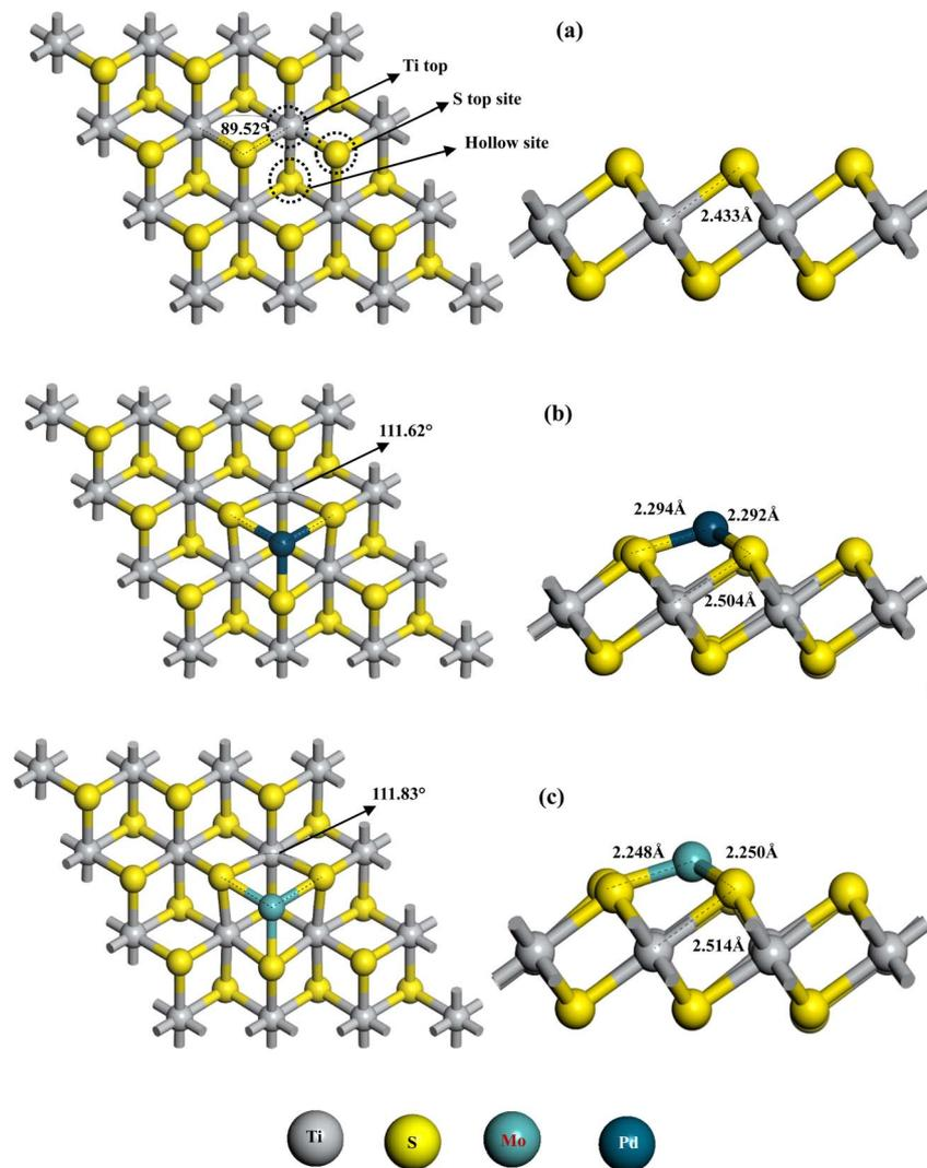
Fig. 2 (a) Optimized  $\text{TiS}_2$  monolayer showing three possible decoration sites, (b and c) most energetically favorable Pd-decorated  $\text{TiS}_2$  and Mo-decorated  $\text{TiS}_2$  monolayers, respectively.
