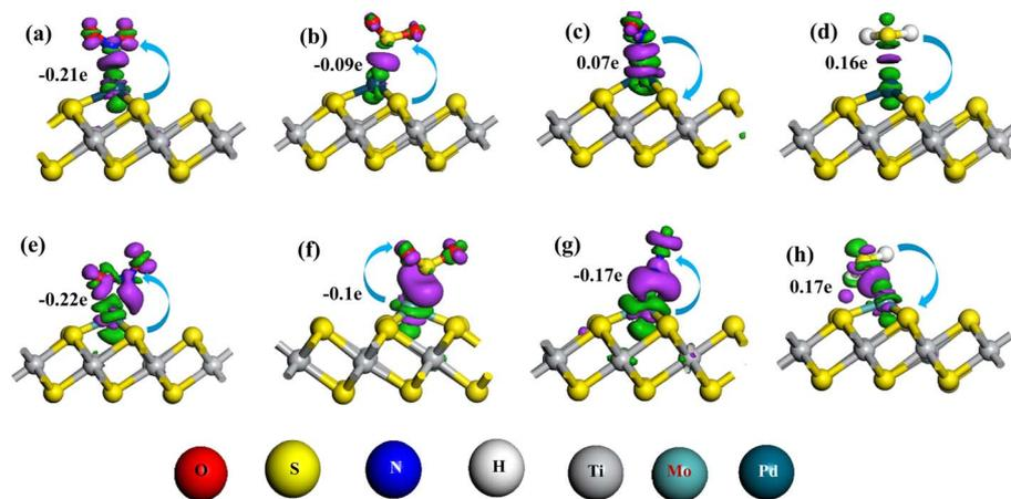
Fig. 5 Charge density difference (CDD) mapping of gas adsorbed systems: (a) NO<sub>2</sub>@Pd/TiS<sub>2</sub>, (b) SO<sub>2</sub>@Pd/TiS<sub>2</sub>, (c) NO@Pd/TiS<sub>2</sub>, (d) H<sub>2</sub>S@Pd/TiS<sub>2</sub>, (e) NO<sub>2</sub>@Mo/TiS<sub>2</sub>, (f) SO<sub>2</sub>@Mo/TiS<sub>2</sub>, (g) NO@Mo/TiS<sub>2</sub>, and (h) H<sub>2</sub>S@Mo/TiS<sub>2</sub>. Here, purple and green colors denote charge accumulation and depletion, respectively.
