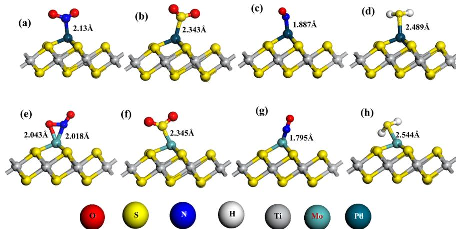
Fig. 4 Most stable optimized systems of adsorbed gas molecules on decorated-TiS<sub>2</sub> monolayers: (a) NO<sub>2</sub>@Pd/TiS<sub>2</sub>, (b) SO<sub>2</sub>@Pd/TiS<sub>2</sub>, (c) NO@Pd/TiS<sub>2</sub>, (d) H<sub>2</sub>S@Pd/TiS<sub>2</sub>, (e) NO<sub>2</sub>@Mo/TiS<sub>2</sub>, (f) SO<sub>2</sub>@Mo/TiS<sub>2</sub>, (g) NO@Mo/TiS<sub>2</sub>, and (h) H<sub>2</sub>S@Mo/TiS<sub>2</sub>.
