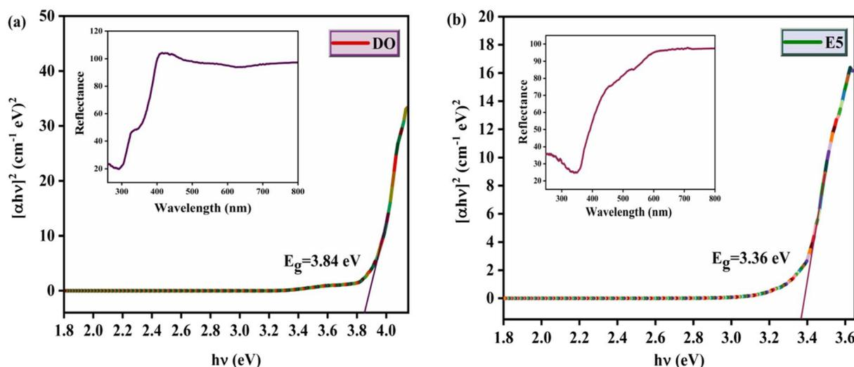
Fig. 7 (a): Tauc plot of DO with the inset displaying its resultant DR spectra. (b): Tauc plot of the E5 [Eu(DO)<sub>3</sub>phen] sample with the inset displaying its resultant DR spectra.
