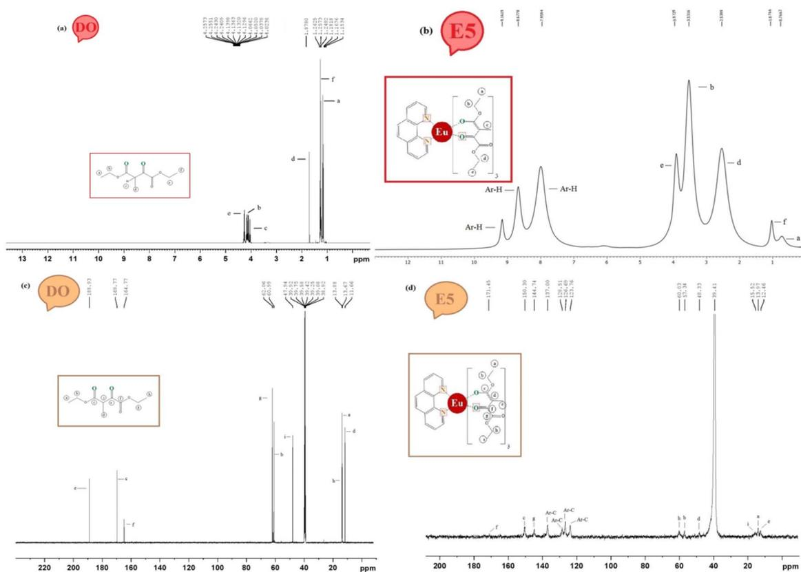
Fig. 4 (a):  $^1\text{H}$  NMR signals (in ppm) of DO. (b):  $^1\text{H}$  NMR signals (in ppm) of E5  $[\text{Eu}(\text{DO})_3\text{phen}]$ . (c):  $^{13}\text{C}$  NMR signals (in ppm) of DO. (d):  $^{13}\text{C}$  NMR signals (in ppm) of E5  $[\text{Eu}(\text{DO})_3\text{phen}]$ .
