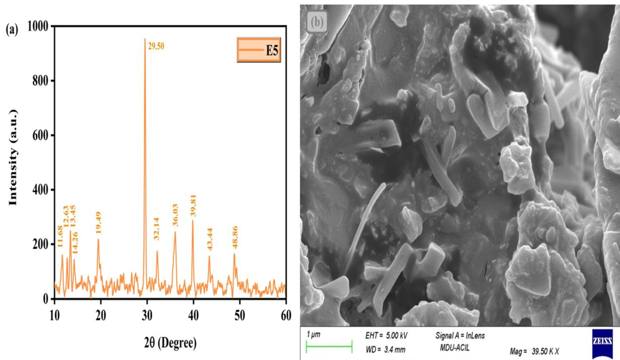
Fig. 2 (a): Powder X-ray diffraction pattern of E5 [Eu(DO)<sub>3</sub>phen]. (b) FESEM micrograph of E5 [Eu(DO)<sub>3</sub>phen].
