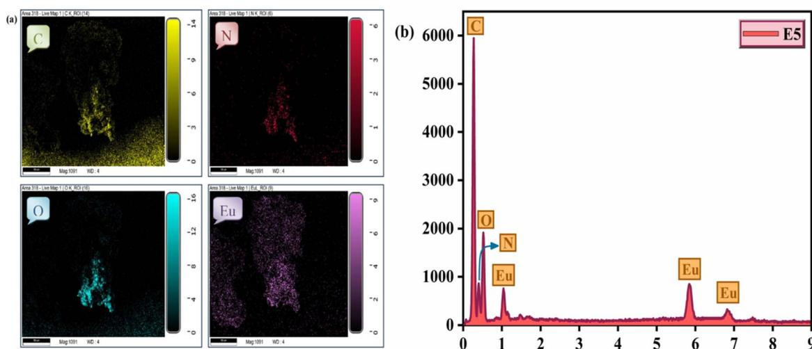
Fig. 1 (a) EDAX mapping displaying the elements Eu, N, C and O of E5 [Eu(DO)<sub>3</sub>phen]. (b): EDAX spectrum of E5 [Eu(DO)<sub>3</sub>phen].
