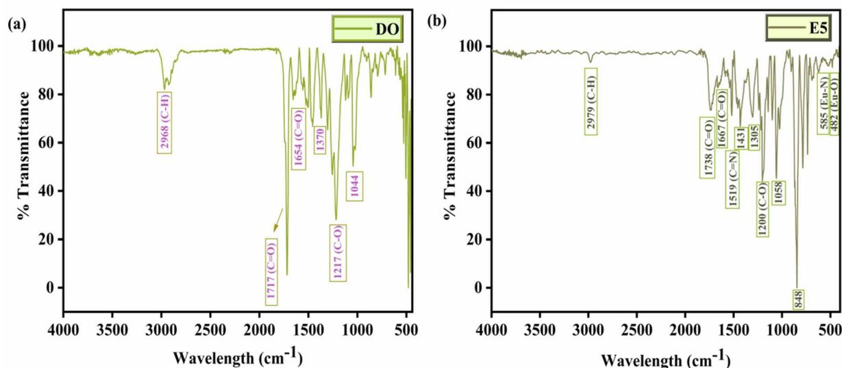
Fig. 3 (a): FT-IR window (in  $\text{cm}^{-1}$ ) of DO. (b): FT-IR window (in  $\text{cm}^{-1}$ ) of E5  $[\text{Eu}(\text{DO})_3\text{phen}]$ .
