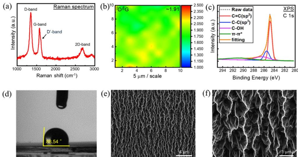
**Fig. 1** (a) Raman spectrum of the as-synthesized graphene. (b) Spatial Raman mapping of the  $I_D/I_G$  ratio with a mean value of about 1.91. (c) XPS spectrum of carbon 1s with both raw data and fitted curves. (d) Contact angle study on the graphene surface. (e) SEM image of the as-synthesized 3D graphene on copper foil. (f) Magnified SEM image to display 3D structure.
