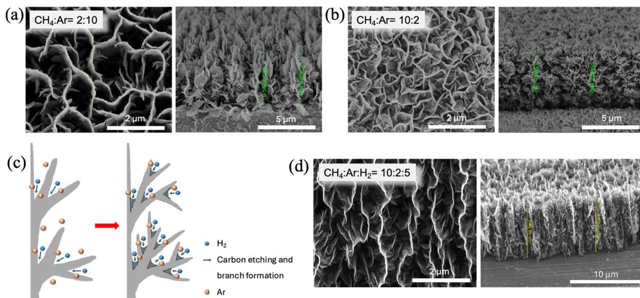
**Fig. 2** (a) FIB images of PECVD-grown 3D graphene under Ar-rich condition with cross-sectional view on the right panel. (b) Image of 3D graphene with low argon growth condition. (c) Schematic of the 3D graphene growth mechanism with additional  $H_2$  introduced. (d) FIB image of the optimized 3D graphene, grown with a  $CH_4 : Ar : H_2$  ratio of 10 : 2 : 5.
