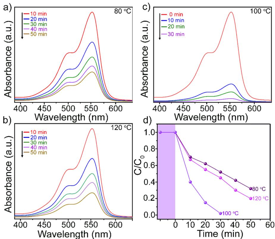
Fig. 2 The absorption spectra of RhB aqueous solution were measured over time using  $\beta$ -FeOOH catalyst produced at three different temperatures: (a) 80 °C, (b) 100 °C, and (c) 120 °C, respectively and (d) the related degrading efficiency curves.
