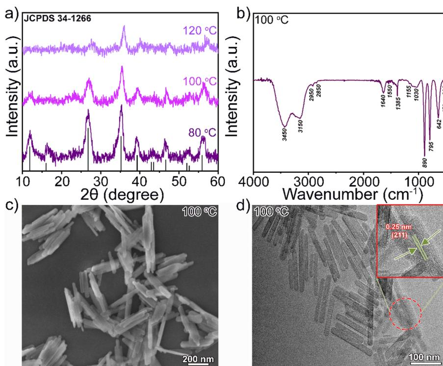
Fig. 1 (a) X-ray diffraction (XRD) spectra taken from the  $\beta$ -FeOOH nanorods synthesized at various reaction temperatures. (b) FTIR spectra analysis (c) Scanning Electron Microscopy (SEM), and (d) Transmission Electron Microscopy analysis of  $\beta$ -FeOOH nanorods. The inset in (d) displays HRTEM analysis of the nanorods.
