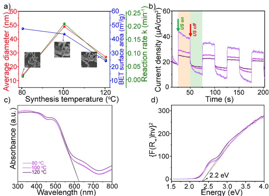
Fig. 3 (a) The mean diameter and surface area of  $\beta$ -FeOOH catalyst synthesized at various temperatures are plotted, with corresponding SEM images shown in the insets. (b) Transient tribocurrent density-time analysis of optimized  $\beta$ -FeOOH catalyst. (c) UV-vis spectra analysis of  $\beta$ -FeOOH catalyst at different temperature, and (d) the corresponding band gap analysis.
