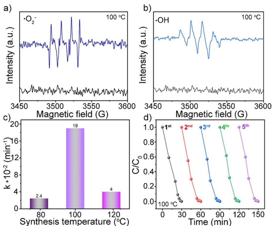
Fig. 4 (a and b) EPR spectrum analysis for detection of  $\cdot\text{O}_2^-$  detection, and  $\cdot\text{OH}$  respectively. (c and d) comparison analysis of the reaction rate constant of  $\beta$ -FeOOH synthesized at different temperatures, and stability analysis for the degradation of RhB, respectively.
