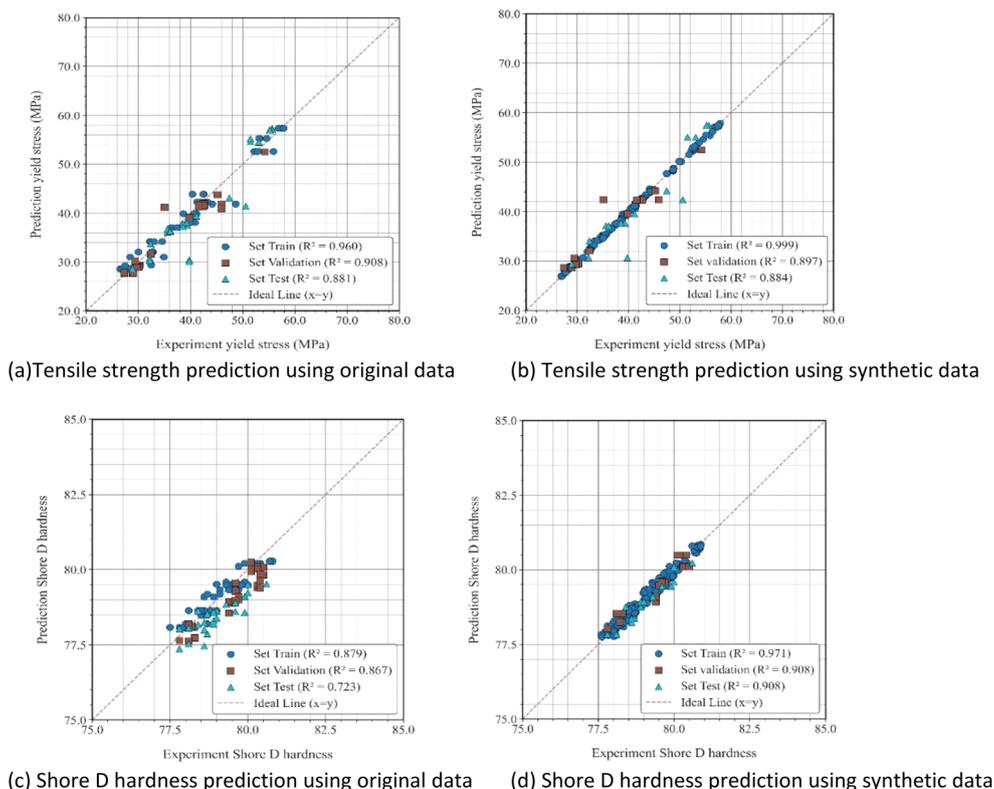
Fig. 7 Comparison of predicted and experimental values for tensile strength and Shore D hardness using original and synthetic datasets. (a) Tensile strength prediction using original data (b) tensile strength prediction using synthetic data (c) Shore D hardness prediction using original data (d) Shore D hardness prediction using synthetic data.
