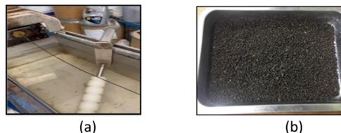
Fig. 3 Extruded bio-composite materials at different processing stages: (a) continuous strands from twin-screw extrusion; (b) pelletized granules after mechanical grinding.
