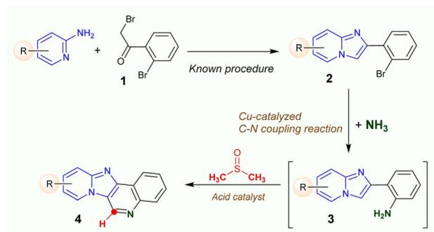
Scheme 2 Synthetic route to prepare pyrido[2',1':2,3]imidazo[4,5-c]quinoline derivatives.
