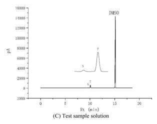
Fig. 3 Gas chromatogram of blank solvent (A), standard solution (B) and test solution (C). (1) Methanol (2) dichloromethane (3) ethyl acetate (4) tetrahydrofuran (5) isopropyl acetate (6) triethylamine (7) *n*-heptane (8) *N*,*N*-dimethylformamide.
