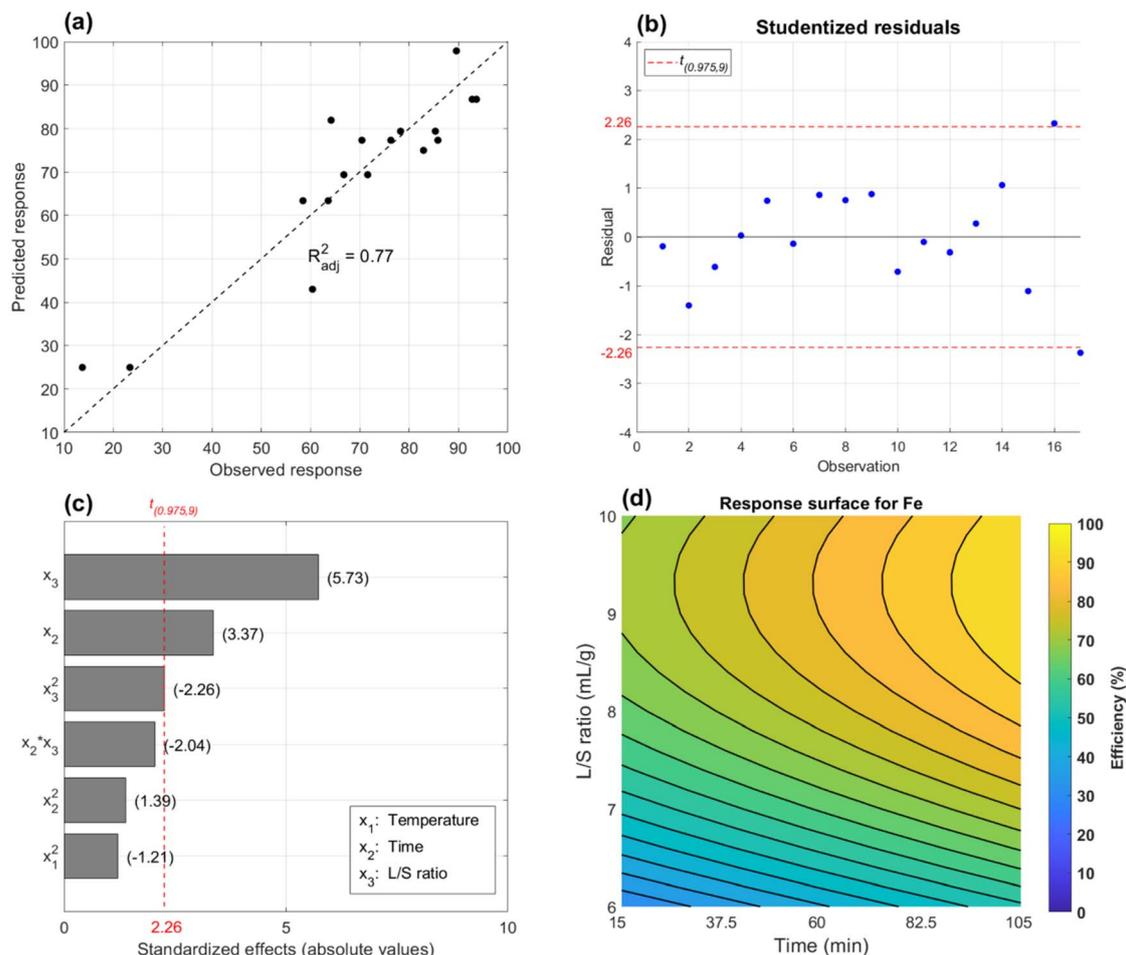
Fig. 3 Regression model diagnostics and response surface for leaching of Fe. Predicted versus observed responses with adjusted  $R^2$  (a), standardized effects and significance of regression parameters (b) and studentized residuals vs. a  $t$ -distribution with 95% confidence (c) for the model in eqn (12). For the same model but including only significant parameters  $x_2$ ,  $x_3$  and  $x_3^2$ , a contour plot of the response surface (d).
