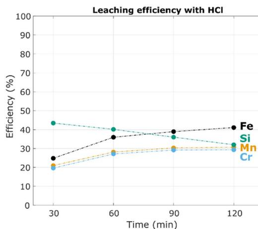
Fig. 6 Leaching efficiencies (%  $E_{s,M}$ ) for grinding swarf (60.40% Fe, 0.80% Mn, 0.16% Cr, 0.17% Si) in 34% HCl at 60 °C with a liquid to solid ratio (L/S) of 3 mL g<sup>-1</sup>.
