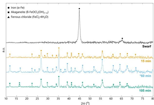
Fig. 5 XRD patterns of grinding swarf and leaching residues from DOE experiments 1 (15 min), 3 (105 min) and 16 (\*60 min). In all three experiments  $L/S = 6 \text{ mL g}^{-1}$ . \* Experiment 16 was conducted at  $40^\circ\text{C}$  contrary to 1 and 3 which were conducted at  $20^\circ\text{C}$ .
