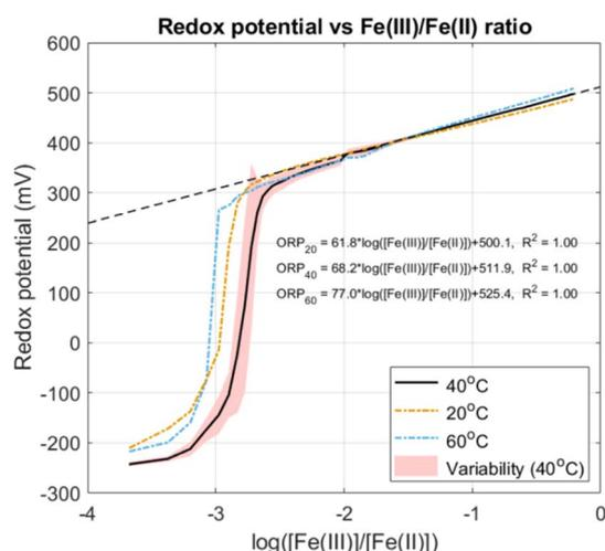
**Fig. 2** Measurement of redox potential for [Fe(III)]/[Fe(II)] ratios at 20 °C, 40 °C and 60 °C and constant total [Fe] = 200 g L<sup>-1</sup>. Experiments at 40 °C were performed in triplicate and the line represents average values with standard deviations visualized by the shaded area. Linear regression was done for all instances in the range log([Fe(III)]/[Fe(II)]) > -2.
