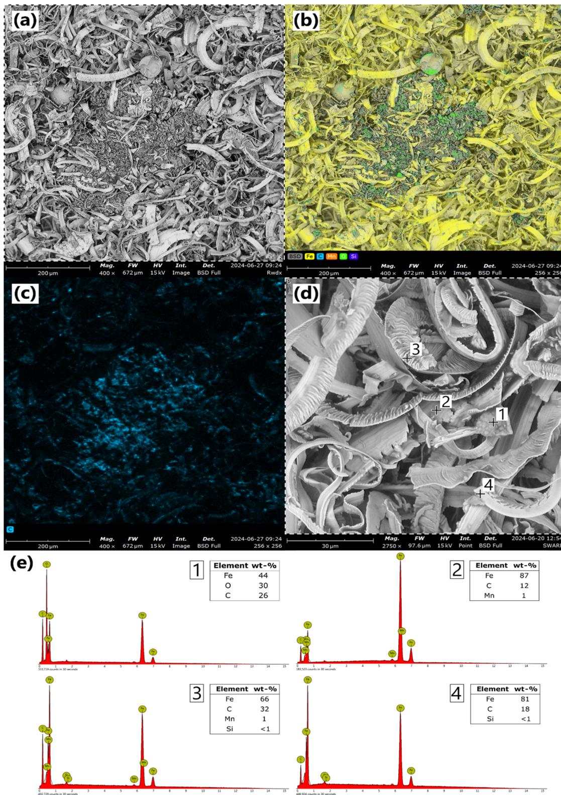
Fig. 1 Backscatter electron SEM image of an oxide cluster at 400 $\times$  magnification (a) with a corresponding EDS elemental map (b), and carbon mapping (c). A typical image of the swarf shavings at 2750 $\times$  magnification (d) with corresponding EDS spot analysis at selected locations (e).
