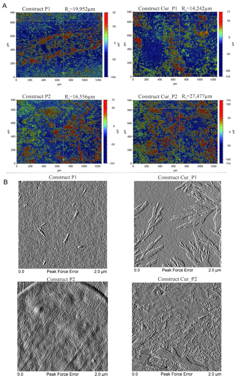
Fig. 7 (A) Profilometric 3D surface maps of Construct P1, Construct Cur\_P1, Construct P2, and Construct Cur\_P2 showing microscale roughness distribution. (B) AFM Peak Force Error images presenting nanoscale topographical features of the same constructs.
