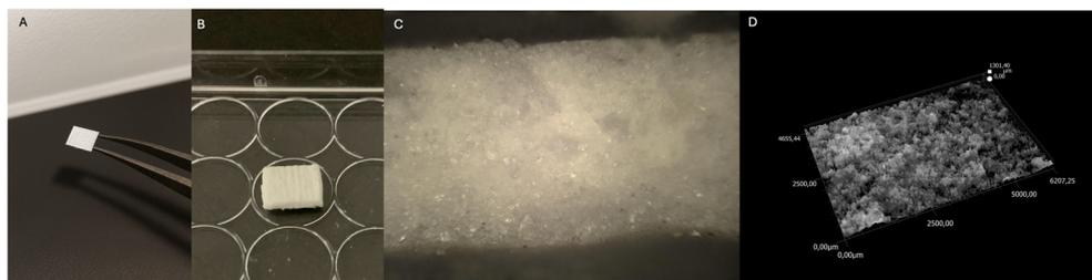
**Fig. 1** Optical images of as printed structures (A and B), (C) cross-section image magn. 500 $\times$ , (D) 3D surface reconstruction of the cross-section surface. Surface topography images of as printed construct were recorded using the digital optical microscope (VHX-7000, Keyence, Japan) with a DIC (VH-Z100UT) varifocal lens for roughness profile measurement and creating 3D model of the surface at magnification of 500 $\times$ .
