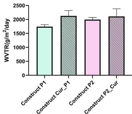
Fig. 10 The water vapor transmission rate coefficients for the printed biomaterials: Construct P1, Construct Cur\_P1, Construct P2, Construct Cur\_P2. No statistically significant differences were observed between the tested samples ( $p > 0.05$ ).
