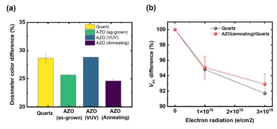
Fig. 4 Electron radiation-shielding performance of AZO-coated quartz glass depending on post-process treatment. (a) Color difference of dosimetry with different AZO-coated glass after simulated electron radiation with an energy of 1.2 MeV and fluency of  $1 \times 10^{15} \text{ e}^- \text{ cm}^{-2}$ ; (b) change in  $V_{oc}$  under different electron beam fluences using AZO-coated glass.
