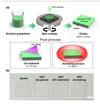
Fig. 1 Process for fabricating radiation-resistant glass by coating AZO thin film. (a) Schematic illustration of the AZO spin coating and posttreatment processes on the quartz glass substrate. (b) Digital image of the bare quartz, the as-grown AZO, UV-treated AZO, and annealed AZO-coated quartz substrates.
