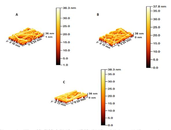
Fig. 3 AFM topography of (A) neat PCL; (B) PCL-0.4%AgNPs; and (C) PCL-1%AgNPs scaffolds. Increased AgNPs concentration correlates with elevated surface roughness and greater topographical heterogeneity across the scaffold surface.
