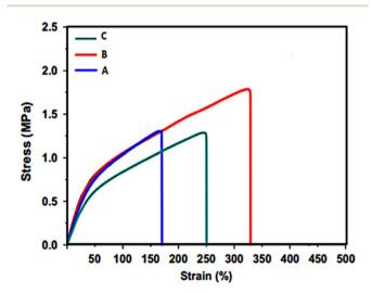
Fig. 5 Tensile stress-strain curves of (A) neat PCL; (B) PCL-0.4% AgNPs; and (C) PCL-1%AgNPs scaffolds. Curves illustrate variations in stiffness and elongation as a function of nanoparticle concentration, with increased modulus at moderate Ag content and decreased mechanical performance at higher loading.
