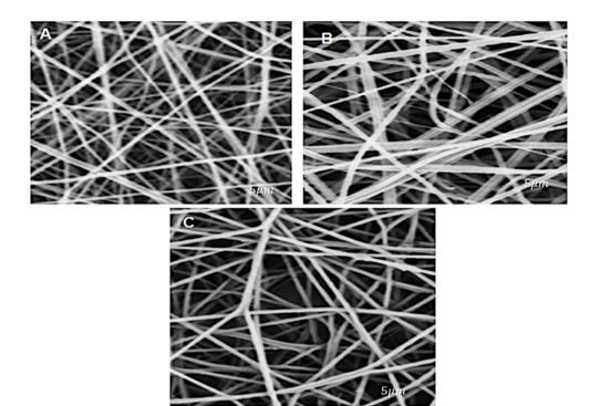
Fig. 2 SEM images of (A) neat PCL; (B) PCL-0.4%AgNPs; and (C) PCL-1%AgNPs scaffolds.
