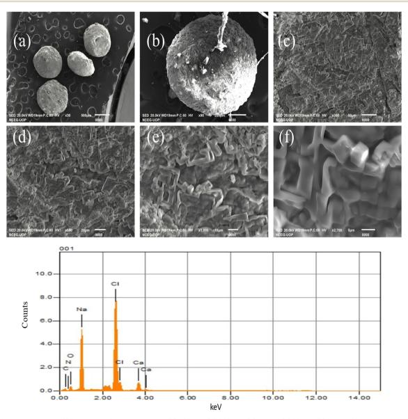
Fig. 3 (A) SEM images of Alg/CSM-loaded CIP microspheres (a)  $500 \mu m$ , (b)  $200 \mu m$ , (c)  $50 \mu m$ , (d)  $20 \mu m$ , (e)  $10 \mu m$ , (f)  $5 \mu m$ , and EDX spectrum (B) showing the elemental composition of the ciprofloxacin microspheres.
