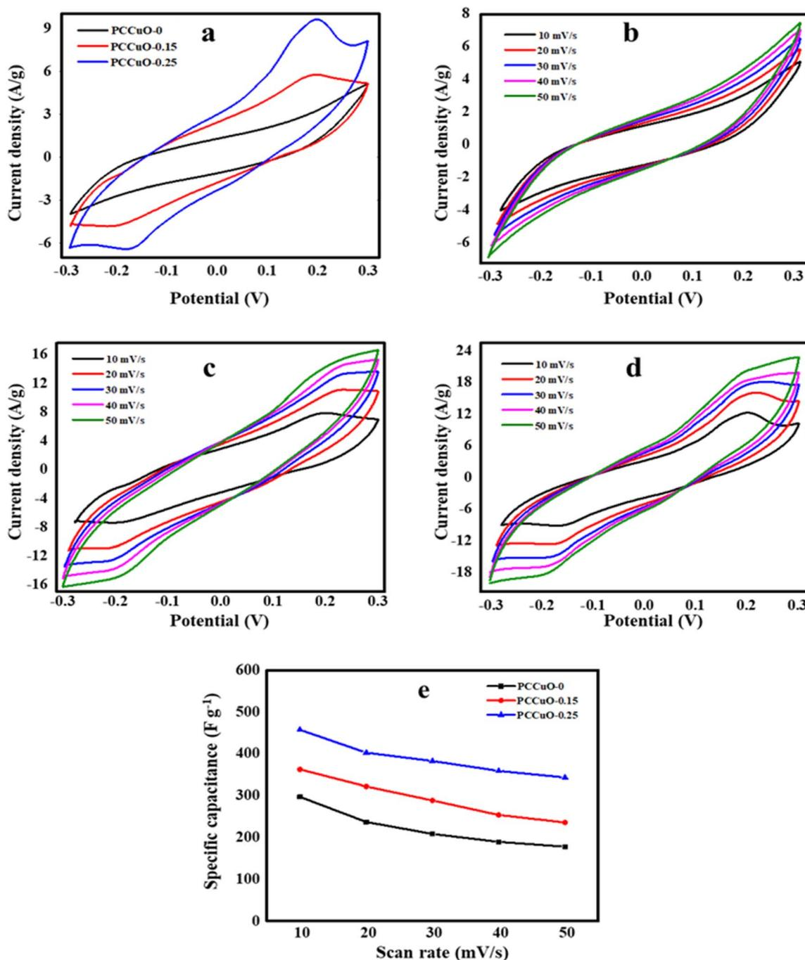
Fig. 6 (a) CV curves of PCCuO-0, PCCuO-0.15 and PCCuO-0.25 electrodes at a scan rate of  $10 \text{ mV s}^{-1}$ ; CV curves of (b) PCCuO-0, (c) PCCuO-0.15, and (d) PCCuO-0.25 at scan rates from 10 to  $50 \text{ mV}^{-1}\text{s}$ ; and (e) variation of specific capacitance with different scan rates from 10 to  $50 \text{ mV s}^{-1}$ .
