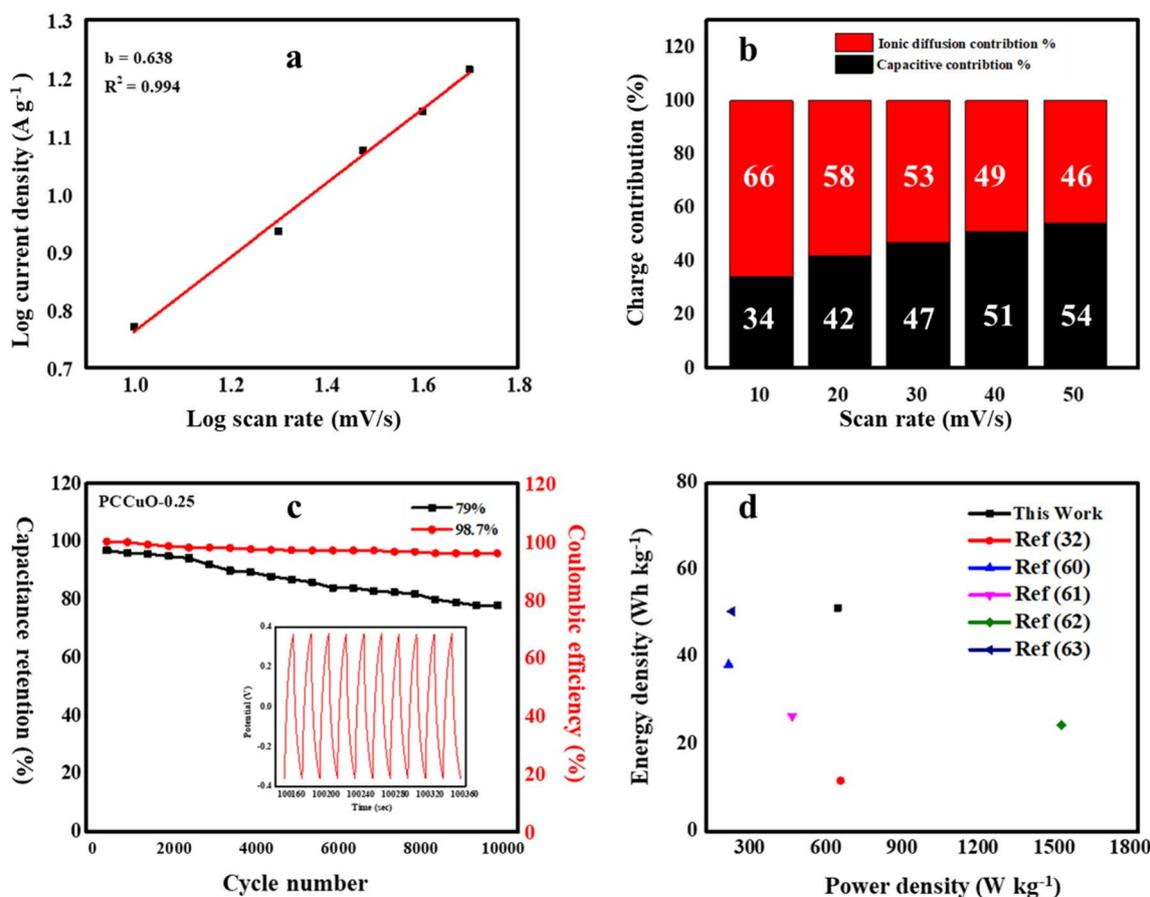
Fig. 10 (a)  $\log(I_p)$  vs.  $\log(v)$  plot; (b) charge contribution of the PCCO-0.25//PCCuO-0.25 SSC; (c) the capacitance retention and coulombic efficiency of the PCCuO-0.25//PCCuO-0.25 SSC at a CD of  $3$   $\text{A g}^{-1}$  (inset: the last 10 cycles of the GCD curve); and (d) comparison of the energy densities of the PCCuO-0.25//PCCuO-0.25 SSC with the previous works.
