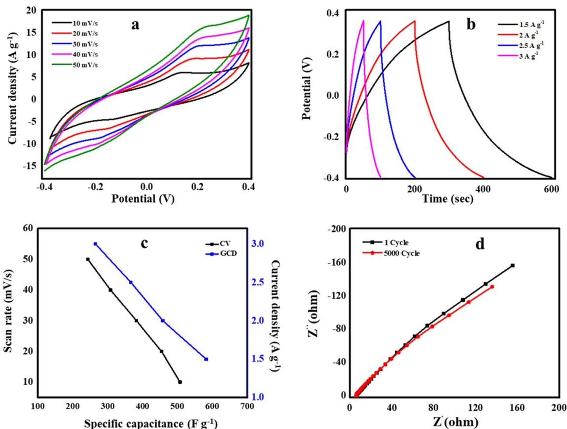
**Fig. 9** (a) CV curve of the PCCuO-0.25 SSC device at various scan rates, (b) GCD curve of the PCCuO-0.25 SSC device at various CDs, (c) comparison of  $C_{sp}$  at different scan rates and CDs for CV and GCD, respectively, and (d) Nyquist plots of the PCCuO-0.25 SSC device for the 1st and 5,000th cycles.
