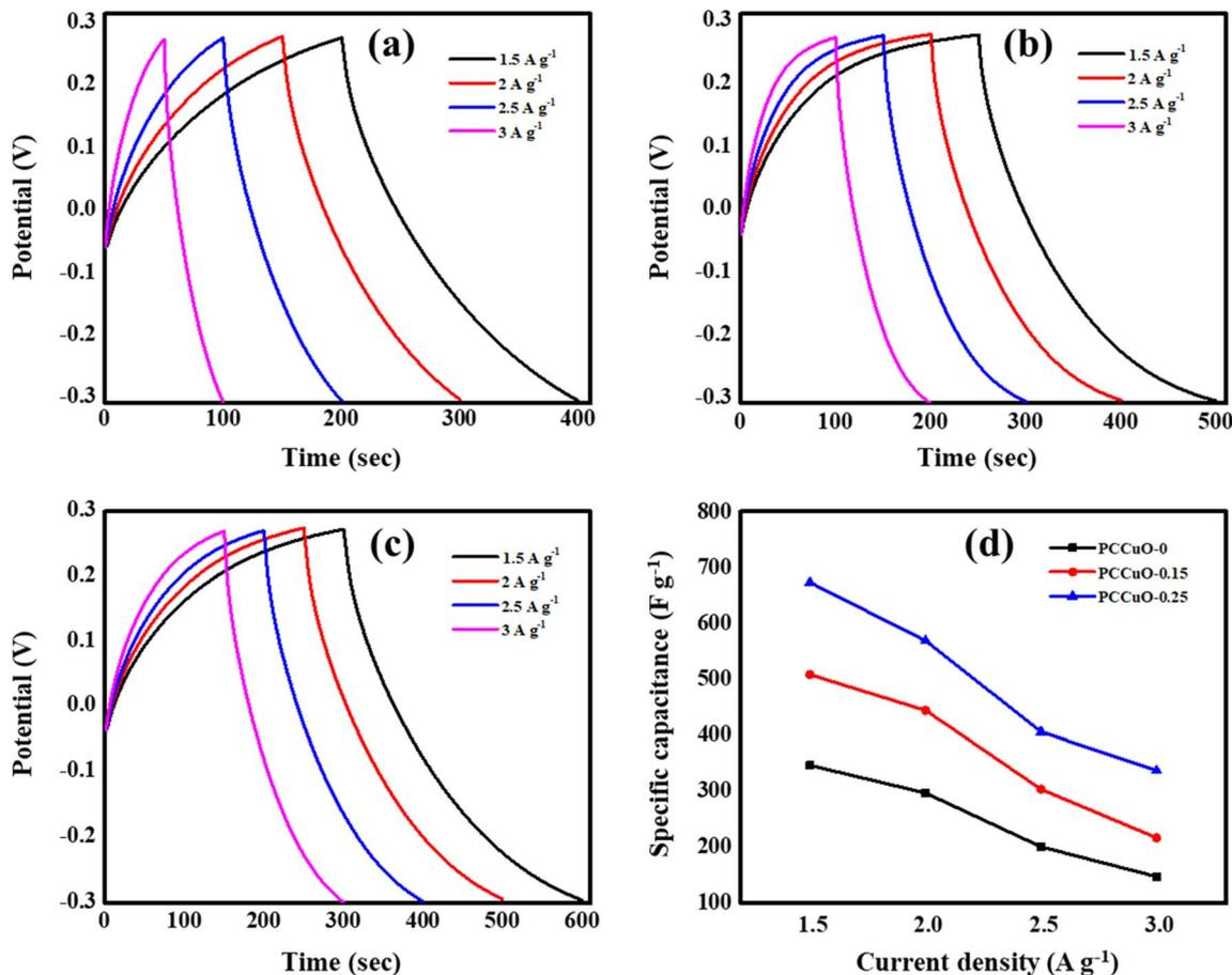
Fig. 7 GCD curves for the (a) PCCuO-0, (b) PCCuO-0.15, and (c) PCCuO-0.25 nanocomposites at varying current densities from 1.5 to 3 A g<sup>-1</sup>; and (d) variation of specific capacitance with CD.
