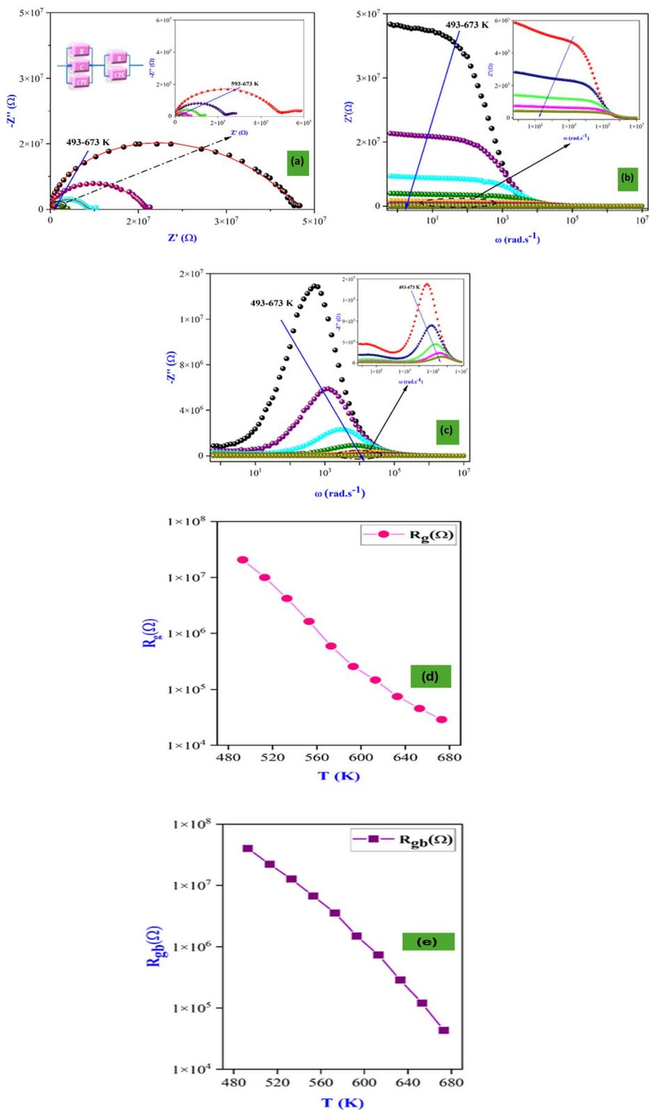
Fig. 3 Nyquist plots (a), the frequency dependence of the real part ( $Z'$ ) (b), imaginary part ( $Z''$ ) of the complex electrical impedance (c), the dependence resistances of grain ( $R_g$ ) (d) and grains ( $R_{gb}$ ) at different temperatures of  $\text{Li}_3\text{Mg}_2\text{NbO}_6$  (e).
