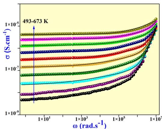
Fig. 4 The variation of ( $\sigma$ ) versus ( $\omega$ ) at different temperatures of  $\text{Li}_3\text{Mg}_2\text{NbO}_6$ .
