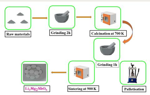
Fig. 1 Process flow chart for the solid-state synthesis of Li<sub>3</sub>Mg<sub>2</sub>NbO<sub>6</sub>.
