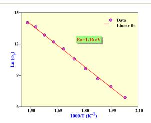
Fig. 11 Dependence of  $ln(\omega_p)$  versus reciprocal temperature for Li<sub>3</sub>Mq<sub>2</sub>NbO<sub>6</sub>.
