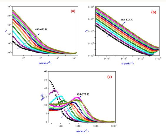
Fig. 8 (a) Frequency-dependent of real part of dielectric constants ( $\epsilon'$ ), (b) imaginary part ( $\epsilon''$ ) and (c)  $tan(\delta)$  at different temperatures of  $Li_3Mg_2NbO_6$ .
