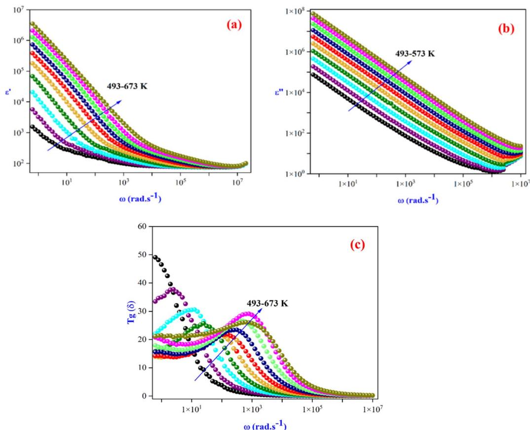
Fig. 8 (a) Frequency-dependent of real part of dielectric constants ( $\epsilon'$ ), (b) imaginary part ( $\epsilon''$ ) and (c)  $\tan(\delta)$  at different temperatures of  $\text{Li}_3\text{Mg}_2\text{NbO}_6$ .
