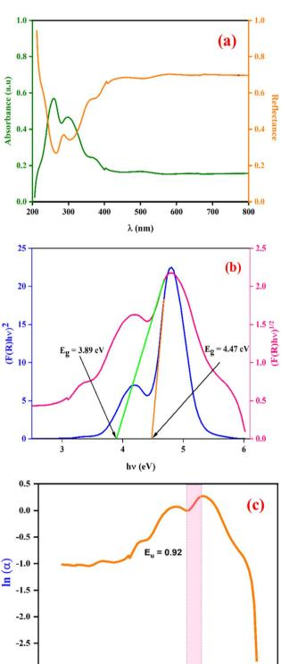
Fig. 13 (a) The UV-visible absorbance spectrum, (b) direct and indirect band gap, (c)  $ln(\alpha)$  as a function of photon energy (eV) for  $Li_3Mg_2NbO_6$ sample
