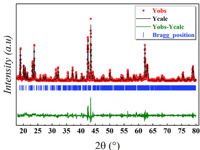
Fig. 2 Rietveld refinement profile carried out through FullProf software of  $\text{Li}_3\text{Mg}_2\text{NbO}_6$ .
