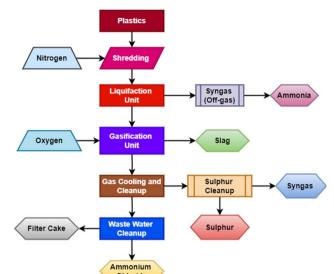
Fig. 4 Process flow diagram for plastic gasification and by-product recovery.
