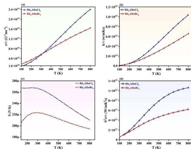
Fig. 9 Thermoelectric factors (a) electrical conductivity ( $\sigma/\tau$ ), (b) thermal conduction ( $k/\tau$ ) (c) Seebeck coefficient ( $S$ ) and (d) power factor of  $\text{Rb}_2\text{AlInX}_6$  ( $X = \text{Cl}, \text{Br}$ ).
