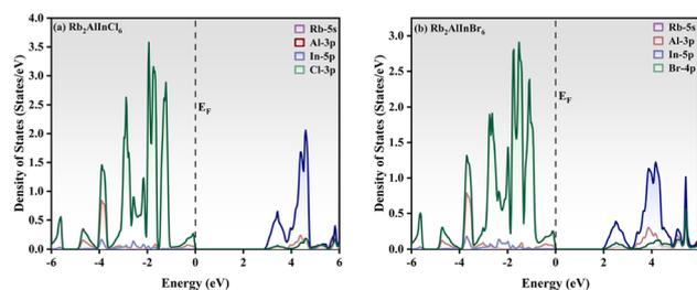
Fig. 6 Partial density of states (PDOS) profile of (a)  $\text{Rb}_2\text{AlInCl}_6$  and (b)  $\text{Rb}_2\text{AlInBr}_6$ .
