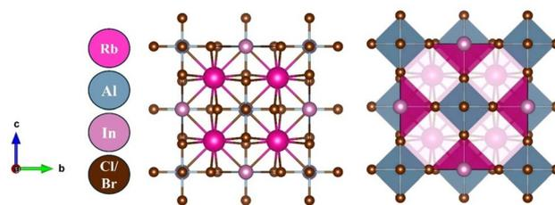
Fig. 1 Crystal structure of  $\text{Rb}_2\text{AlInX}_6$  ( $X = \text{Cl}, \text{Br}$ ).
