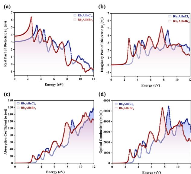
Fig. 7 Optical parameters (a) real  $\epsilon_1(\omega)$  component, (b) imaginary  $\epsilon_2(\omega)$  component, (c) absorption coefficient  $\alpha(\omega)$  and (d) optical conductivity  $\sigma(\omega)$  for  $\text{Rb}_2\text{AlInX}_6$  ( $X = \text{Cl}, \text{Br}$ ).
