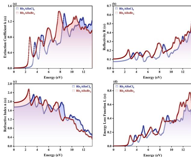
Fig. 8 Optical features of  $\text{Rb}_2\text{AlInX}_6$  ( $X = \text{Cl}, \text{Br}$ ). (a) Extinction coefficient  $k(\omega)$ , (b) reflectivity  $R(\omega)$ , (c) refractive index  $n(\omega)$  and (d) energy loss function  $L(\omega)$ .
