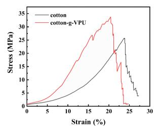
Strain-stress curve of cotton and cotton-q-VPU
