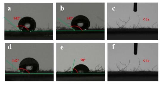
Fig. 7 (a) Cotton-*g*-VPU contact angle before washing. (b) Cotton-PU contact angle before washing. (c) Cotton contact angle. (d) Cotton-*g*-VPU contact angle after washing. (e) Cotton-PU contact angle after washing. (f) Cotton contact angle after washing.
