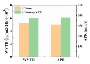
Fig. 8 Water Vapor Transmission Rate (WVTR) and Air Permeability Rate (APR) of cotton and cotton-q-VPU.
