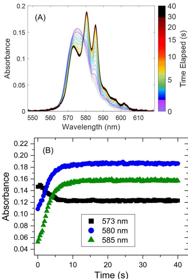
Fig. 4 Results of the *operando* UV/visible absorption spectroscopy of Nd extraction from 2.6 M  $\text{HNO}_3$  by 0.10 M TODGA/*n*-dodecane, monitoring the hypersensitive  $^4I_{9/2} \rightarrow ^4G_{5/2}, ^2G_{7/2}$  absorption bands of Nd(III) at 295 K. (A) Spectra collected from 547–619 nm over 40 s and (B) absorbance changes over time for three of the most prominent wavelengths.
