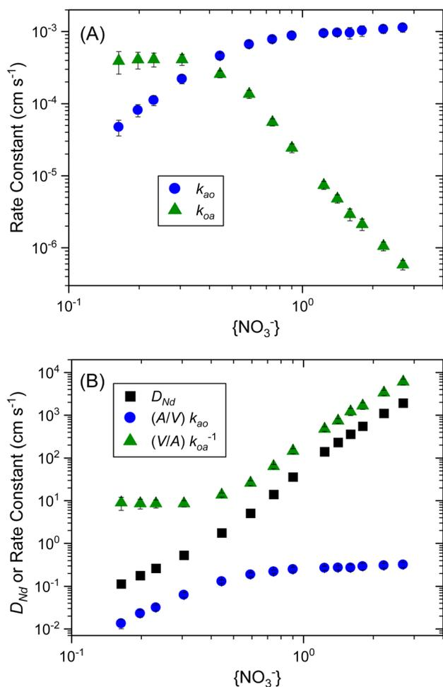
Fig. 6 Acid dependence varying the equilibrium aqueous nitrate anion activity from 0.16–2.69 (0.20–3.0 M HNO<sub>3</sub>) with constant 0.10 M TODGA and 4.9 × 10<sup>-3</sup> M initial aqueous Nd<sup>3+</sup> at 295 K. (A) Pseudo-first order rate constants for extraction (blue circles) and stripping (green triangles). (B) A comparative plot of  $D_{Nd}$ ,  $k_{ao}$  and  $k_{oa}^{-1}$  showing similar trends in the parameters.
