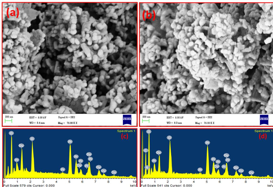
Fig. 4 FESEM images of (a) uncoated, (b) coated with 9 wt% PVP; and EDX spectra: (c) uncoated, (d) coated with 9 wt% PVP  $\text{Dy}_2\text{O}_3/\text{Pr}_2\text{O}_3$  nanocomposites.
