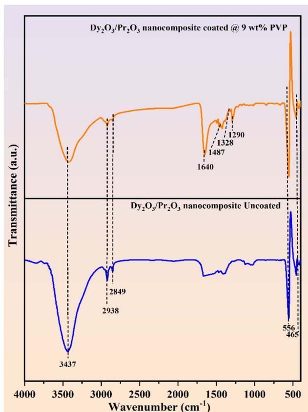
**Fig. 2** FTIR spectra of uncoated and 9 wt% PVP coated Dy<sub>2</sub>O<sub>3</sub>/Pr<sub>2</sub>O<sub>3</sub> nanocomposite.
