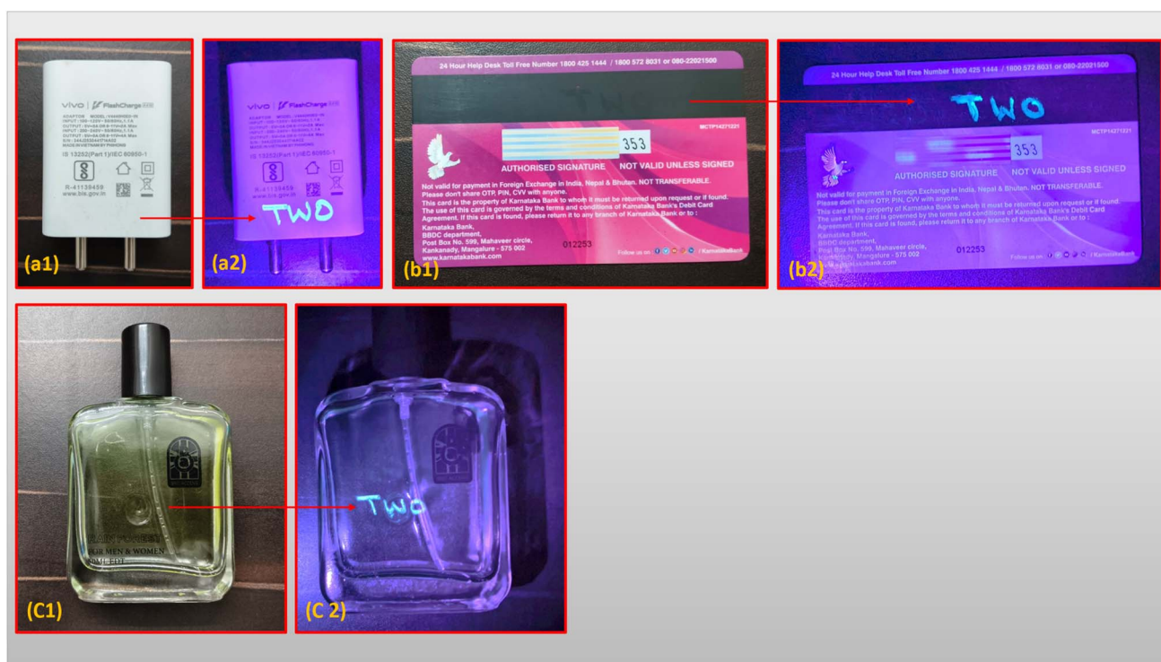
Fig. 8 Anti-counterfeiting labels painted with \text{Dy}_2\text{O}_3/\text{Pr}_2\text{O}_3 nanocomposite coated with 9 wt% PVP ink under visible light (a1–c1) and 365 nm UV light.
