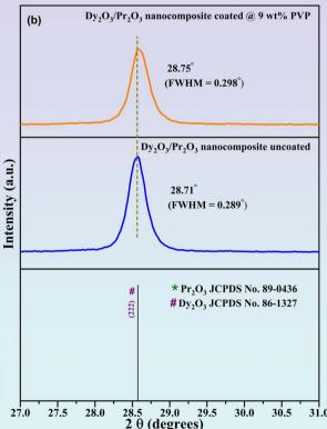
Fig. 1 PXRD patterns of (a) uncoated and 9 wt% PVP coated Dy<sub>2</sub>O<sub>3</sub>/  $Pr_2O_3$  nanocomposite. (b) Enlarged view of PXRD patterns in the  $2\theta$ range 27-31°.
