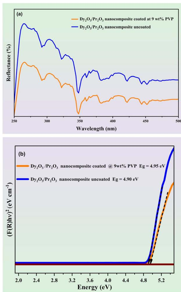
**Fig. 3** (a) UV-Vis diffuse reflectance spectra and (b) band-gap values of uncoated and 9 wt% PVP coated Dy<sub>2</sub>O<sub>3</sub>/Pr<sub>2</sub>O<sub>3</sub> nanocomposite.
