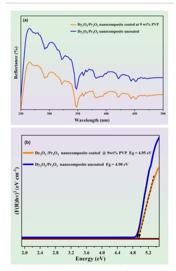
Fig. 3 (a) UV-Vis diffuse reflectance spectra and (b) band-gap values of uncoated and 9 wt% PVP coated  $Dy_2O_3/Pr_2O_3$  nanocomposite.
