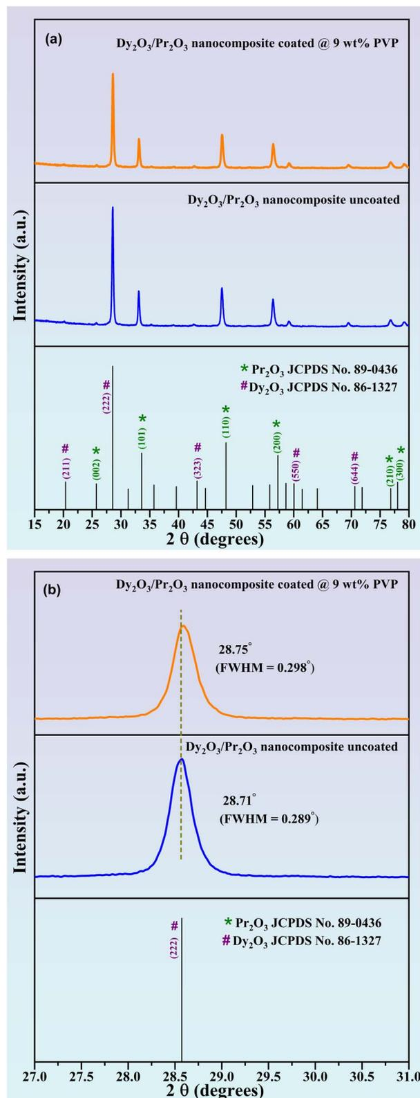
Fig. 1 PXR patterns of (a) uncoated and 9 wt% PVP coated  $\text{Dy}_2\text{O}_3/\text{Pr}_2\text{O}_3$  nanocomposite. (b) Enlarged view of PXR patterns in the  $2\theta$  range 27–31°.
