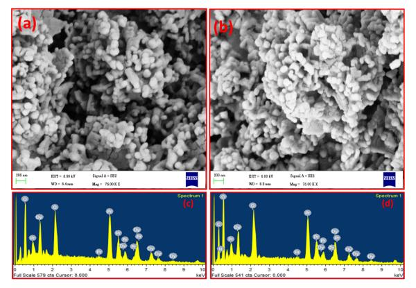
Fig. 4 FESEM images of (a) uncoated, (b) coated with 9 wt% PVP; and EDX spectra: (c) uncoated, (d) coated with 9 wt% PVP Dy<sub>2</sub>O<sub>3</sub>/ Pr<sub>2</sub>O<sub>3</sub> nanocomposites.
