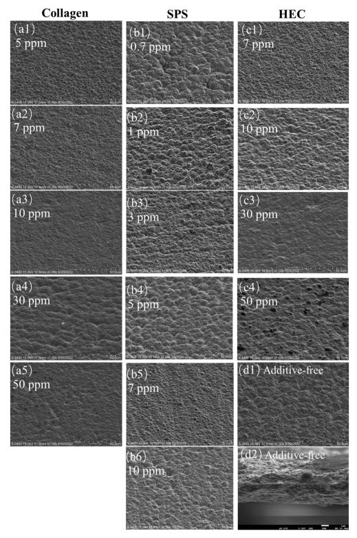
Fig. 2 SEM morphology of the copper foils obtained by electrodeposition at different additives concentrations (a1-a5) collagen; (b1-b6) SPS; (c1-c4) HEC; and (d) additive free.
