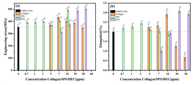
Fig. 5 (a) The elongation of copper foils obtained by electrodeposition at varying concentrations of collagen, SPS, and HEC. (b) The tensile strength of copper foils obtained by electrodeposition at varying concentrations of collagen, SPS, and HEC.
